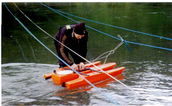
A Greater Wellington staff member testing the new river flow measurement equipment on the Otaki River.
