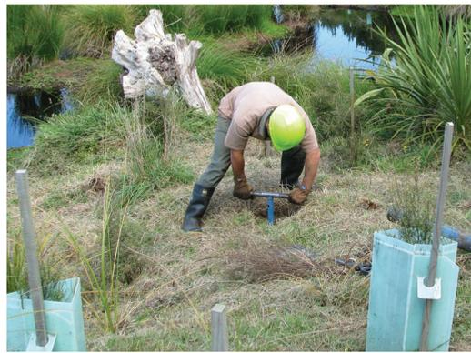
Greater Wellington staff member hand drilling a groundwater level monitoring bore at Te Hapua Wetland at Te Horo on the Kapiti Coast. As outlined in the *Rainfall and river flows* report card, we installed monitoring equipment in the Te Hapua Wetland on the Kapiti Coast to better understand how the wetland system works. The project included drilling two groundwater monitoring bores.
