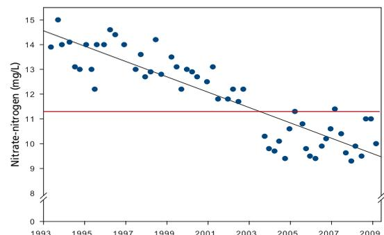
Nitrate-nitrogen concentrations measured over time in a bore north of Otaki. The black line indicates the overall decreasing trend in concentrations. The red line indicates the national drinking water standard (11.3 mg/L).
