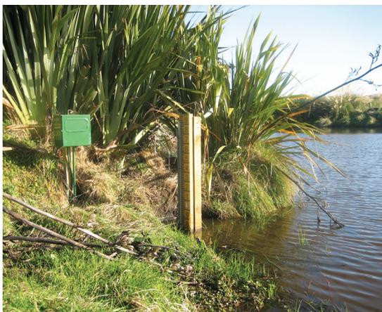
A new monitoring site in the Te Hapua wetland complex. Automatic monitoring equipment records the water level every 15 minutes. The readings are sent to the Greater Wellington office via telemetry, and can be viewed on our website.
