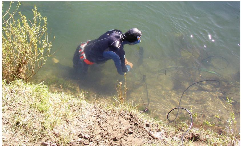
Installing dissolved oxygen monitoring equipment in a river in the Wairarapa. Low river flows may result in low dissolved oxygen concentrations, particularly in small streams with a lot of aquatic plant growth. The dissolved oxygen monitoring results will be taken into account when we recommend minimum flows for small streams.
