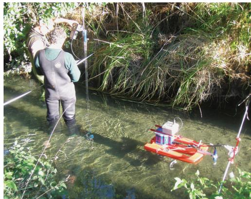
Greater Wellington staff measuring the flow in a stream in the Wairarapa. Small streams can support important values, such as providing habitat for threatened fish species. In some parts of the region, small streams are also used as a source of water for irrigation. In order to set appropriate minimum flow policies, it is important that we collect accurate information about stream flows.
