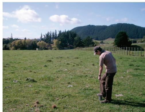
This dairy farm in Otaki is one of our soil quality monitoring sites. At each monitoring site, samples are taken from a depth of 0-10cm using a soil corer (pictured above), tested for various indicators, and the results compared with the optimum range for the soil type and land use. The soil at this site was slightly compacted but nutrient levels were satisfactory.
