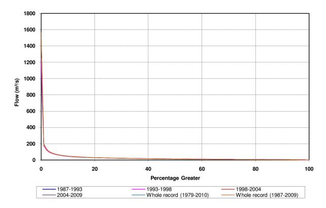
Figure 2.8: Flow distribution over each inter-survey period.
