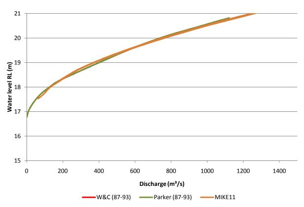
Figure 4.2: Modelled discharge/water level rating curves.
