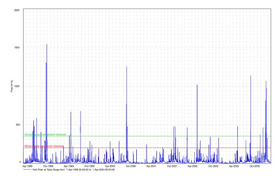
Figure 2.6: Flow record for Hutt River at Taita Gorge 1 April 1998-31 March 2004, including bedload entrainment thresholds.
