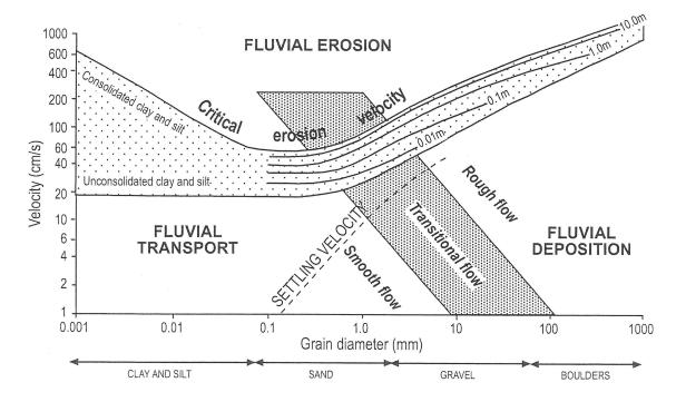
Figure 1.2: Erosion, entrainment, and transport thresholds for different size particles (After Sundborg, 1956).
