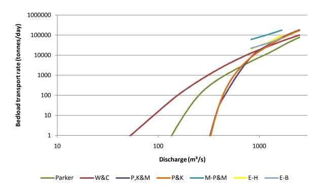
Figure 4.1: Bedload transport rating curves.
