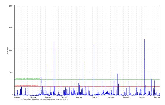
Figure 2.5: Flow record for Hutt River at Taita Gorge 1 August 1993-31 March 1998, including bedload entrainment thresholds.
