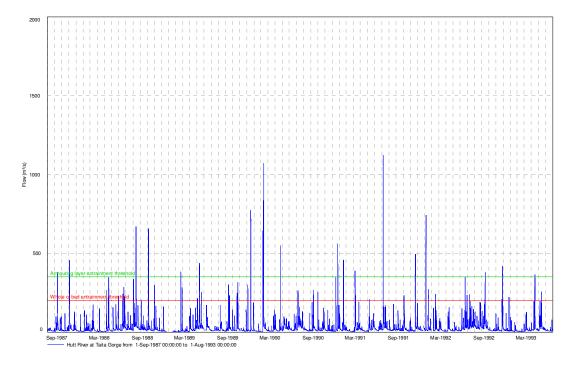
Figure 2.4: Flow record for Hutt River at Taita Gorge 1 Sept 1987-31 July 1993, including bedload entrainment thresholds.
