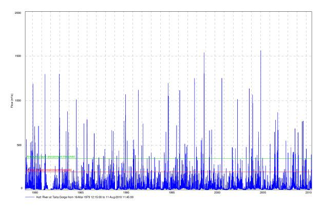
Figure 2.1: Flow record for the Hutt River at Taita Gorge, including two bedload entrainment thresholds (1979-2010).
