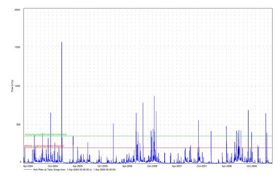
Figure 2.7: Flow record for Hutt River at Taita Gorge 1 April 2004-31 March 2009, including bedload entrainment thresholds.
