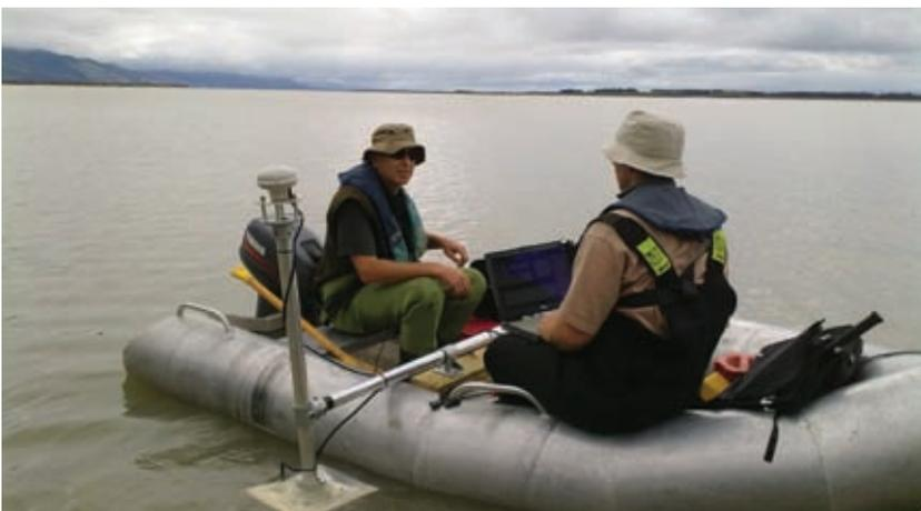
Staff using an echosounder (sonar) during a bathymetric survey in Lake Wairarapa in February. Lake Onoke was also surveyed. A bathymetric survey enables us to measure and map the amount of sediment that has built up over time on the lake bed.
