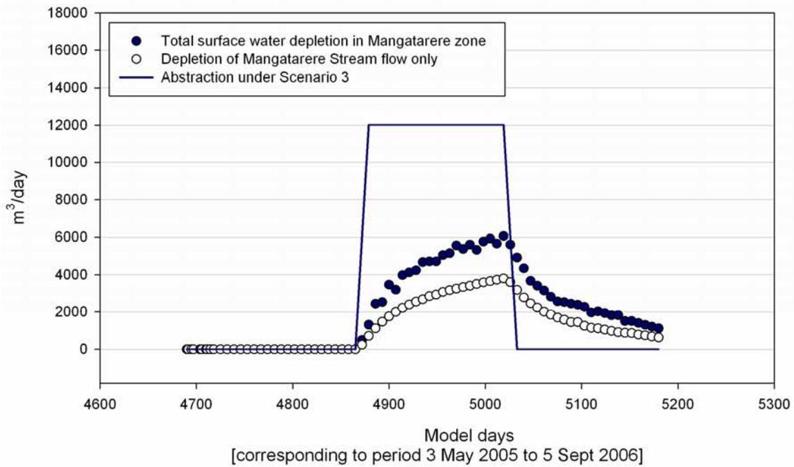
Figure E19: Scenario 3 output – surface water depletion in the Mangatarere zone and in the Mangatarere Stream resulting from pumping an array of synthetic bores located in the Q6 semi-confined aquifer at a rate of 12,000 m<sup>3</sup>/day for 150 days
