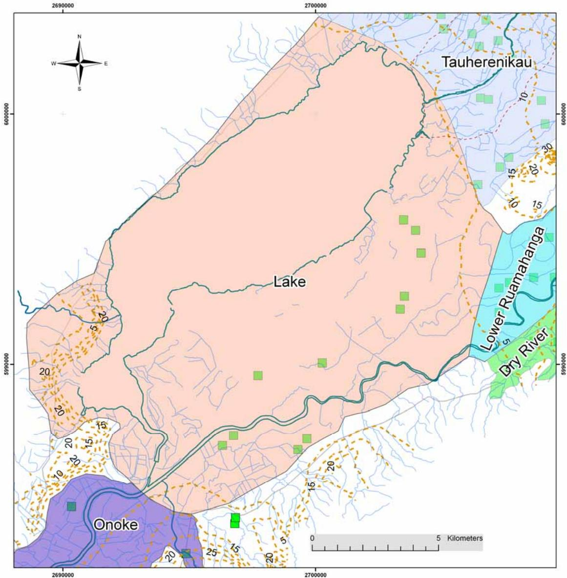
Figure F3: The proposed Lake water management zone showing existing groundwater bores with consented abstraction (green squares), and simulated groundwater flow contours (brown dashed lines at 5 m; contour line following north-easterly lake margin is 5 m amsl). Note there is a very flat hydraulic gradient in this zone and most groundwater throughflow discharges into Lake Wairarapa.
