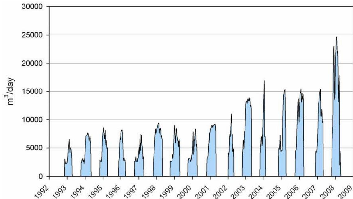
Figure F6: Simulated abstraction in the Lake zone from 12 bores with consented takes peaking at about 25,000 m<sup>3</sup>/day during the 2007/08 irrigation season (most bores were metered weekly during the 2007/08 irrigation season)
