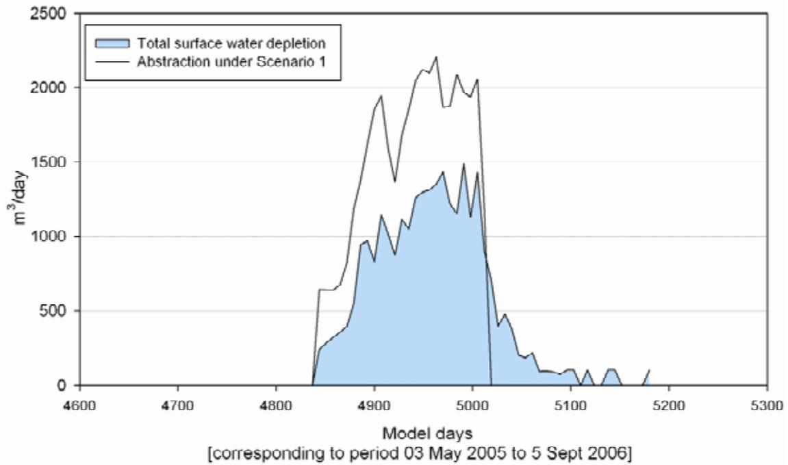
Figure E16: Scenario 1 output – total surface water depletion in the Mangatarere zone from pumping bores with existing consents to abstract that are located in the shallow unconfined aquifers (excluding Q1 deposits)
