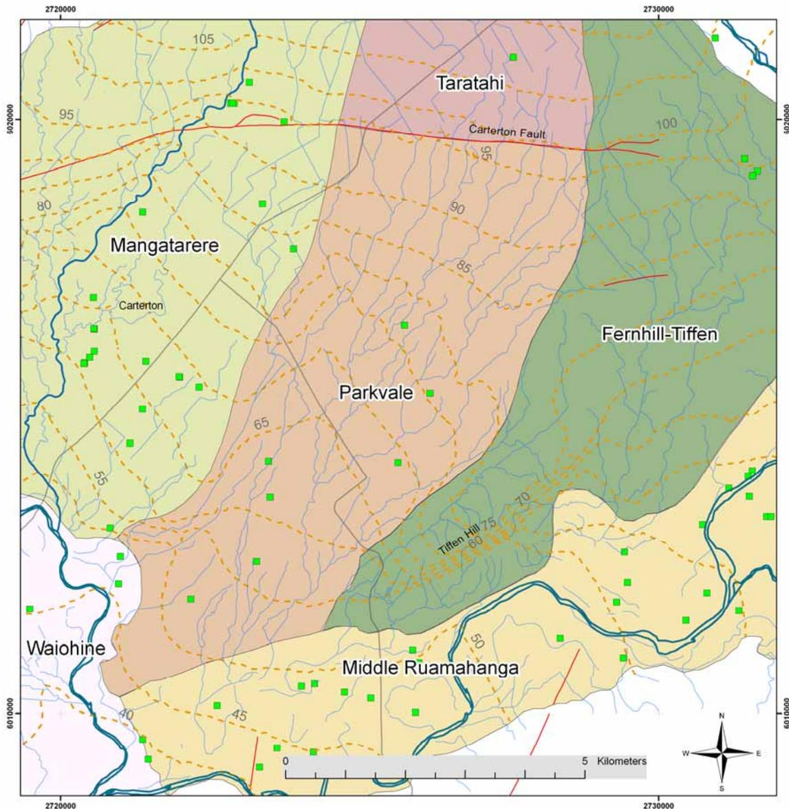
Figure E21: The proposed Parkvale water management zone map showing existing groundwater bores with consented abstraction (green squares) and simulated groundwater flow contours (brown dashed lines at 5 m intervals in metres above mean sea level)
