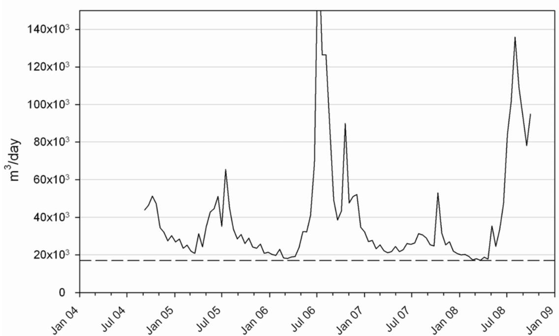
Figure F31: Simulated natural discharge to Featherston springs when there is no groundwater abstraction. Mean low flow is about 17,000 m³/day (200 L/s) and is indicated by the dashed line.
