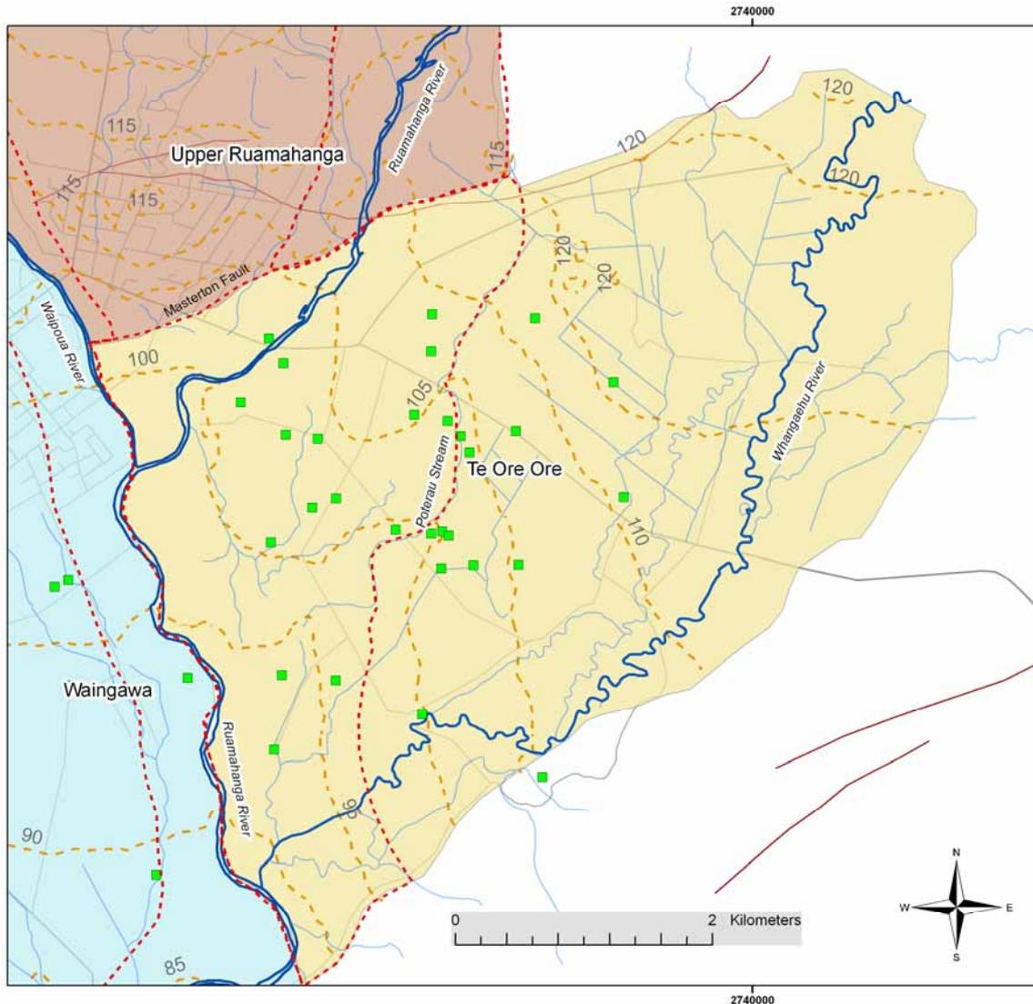
Figure D3: The proposed Te Ore Ore water management zone map showing existing groundwater bores with consented abstraction (green squares) and simulated groundwater flow contours (brown dashed lines, 5 m intervals in metres above mean sea level). The extent of the aquifer system classified as Category A (direct hydraulic connection) is illustrated by the dashed red line.
