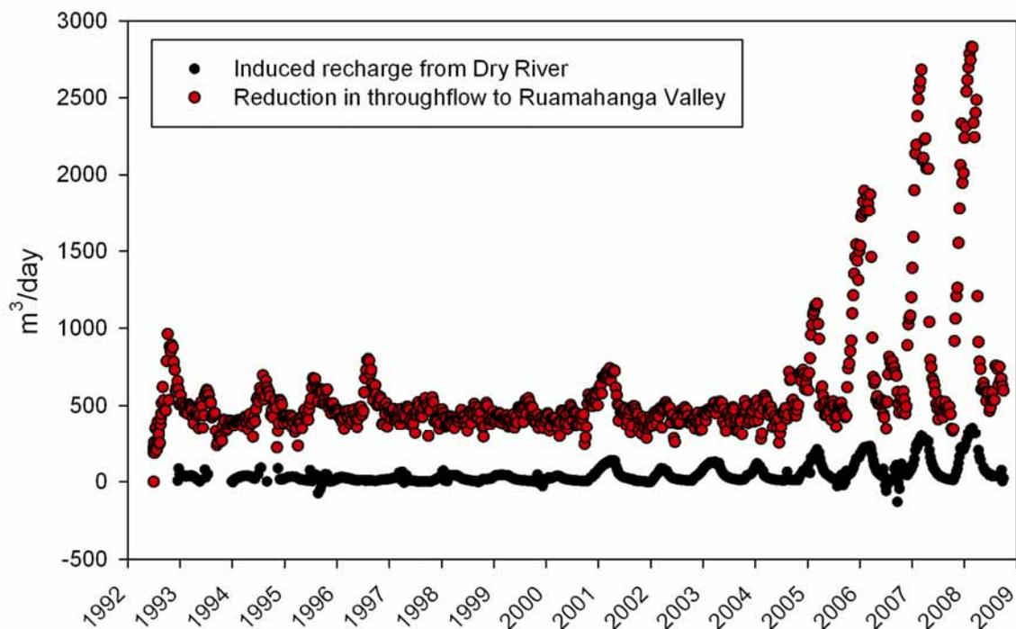
Figure F60: Simulated depletion in throughflow from the Dry River zone across the Martinborough Fault into the Lower Ruamahanga zone, and induced recharge from the Dry River. The throughflow depletion attains about 90% of the abstraction rate. Pumping is occurring in all Lower Valley water management zones during this simulation.
