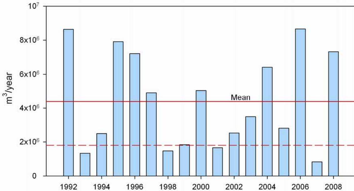
Figure D4: Modelled annual rainfall recharge for the Te Ore Ore zone in the Upper Valley catchment between 1992 and 2008. A mean recharge of  $4.4 \times 10^6 \text{ m}^3/\text{year}$  is indicated as is the lower quartile value of  $1.8 \times 10^6 \text{ m}^3/\text{year}$  (dashed line).
