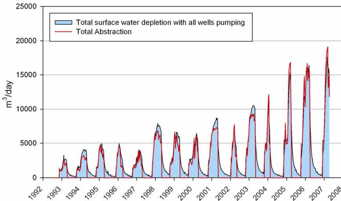
Figure E7: Simulated total surface water depletion resulting from abstraction from all consented bores in the Waiohine water management zone. Effects of groundwater abstraction from adjacent zones are responsible for depletion apparently exceeding pumping rate in some years.
