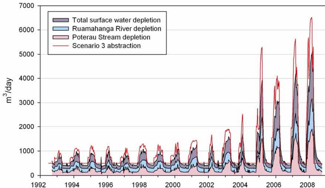
Figure D11: Scenario 3 model results for the period 1992 to 2008 – surface water depletion when pumping from the eastern side of the Te Ore Ore zone. Pumping from model slices 2–4 (ground surface to about 45 m depth)
