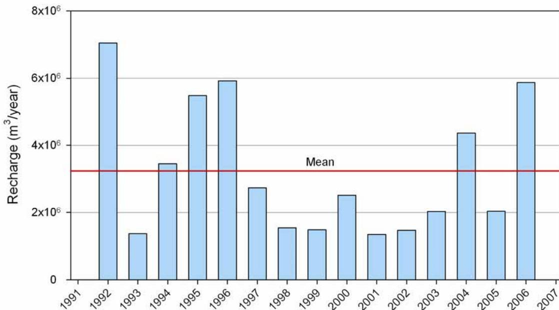
Figure E38: Modelled annual rainfall recharge (1992–2006) for the Fernhill-Tiffen water management (mean recharge of  $3.25 \times 10^6 \text{ m}^3/\text{year}$ )
