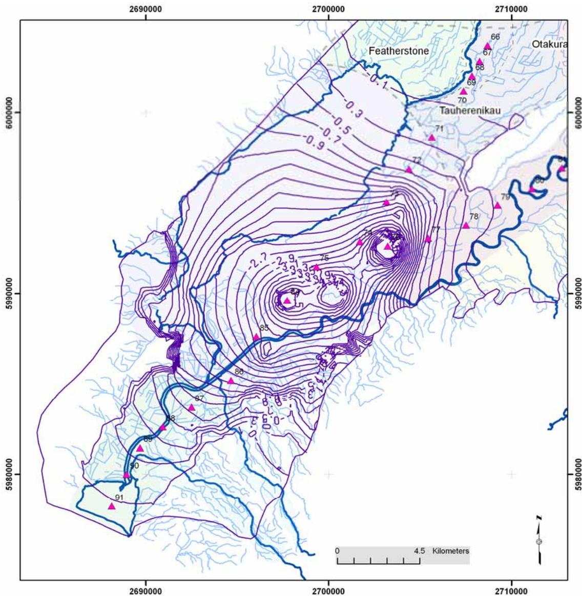
Figure F8: Simulated drawdowns in the confined Q2 aquifer associated with a combined abstraction of 25,000 m<sup>3</sup>/day from 12 bores located in both the Q2 and Q4 aquifers. Output is for model day 5,698 (mid 2007/08 irrigation season). Drawdown contour interval is 0.2 m and the outermost contour denotes 0.1 m of drawdown. Pink numbered triangles are the head observation points used to construct Figure F9.
