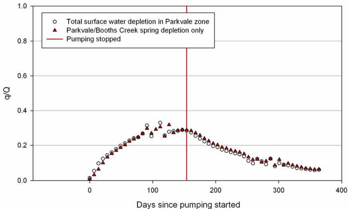
Figure E29: Scenario 1 output – surface water depletion resulting from groundwater abstraction from the unconfined aquifer in the Parkvale zone expressed as the ratio of depletion rate ( $q$ ) and pumping rate ( $Q$ )
