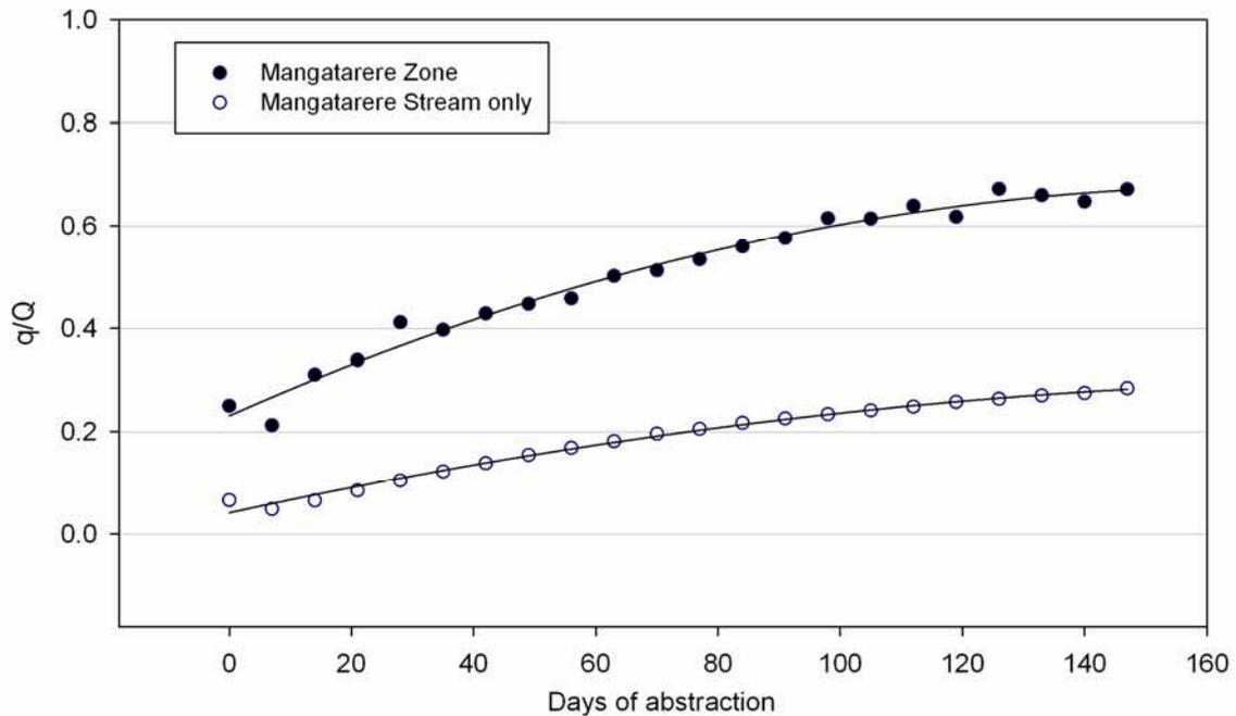
Figure E18: Scenario 2 – ratio of surface water depletion ( $q$ ) to pumping rate ( $Q$ ) for both the Mangatarere zone (total depletion for streams and springs) and Mangatarere Stream only – shallow aquifer abstraction only
