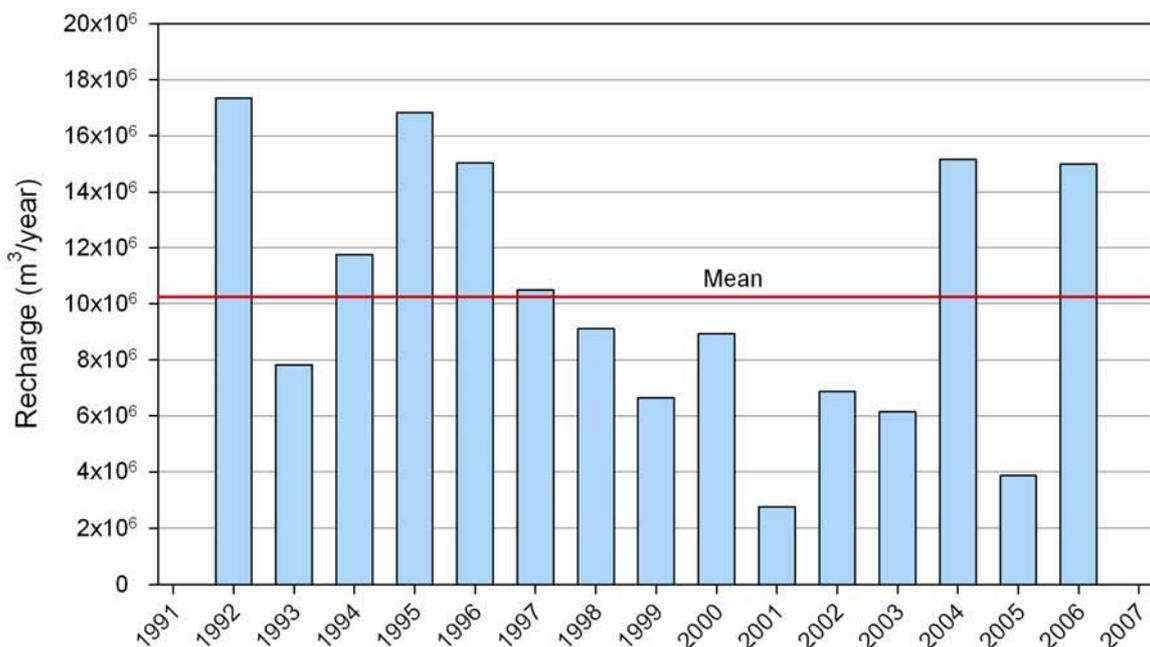
Figure E4: Modelled annual rainfall recharge for the Waiohine zone in the Middle Valley catchment providing a mean recharge of  $10.25 \times 10^6 \text{ m}^3/\text{year}$
