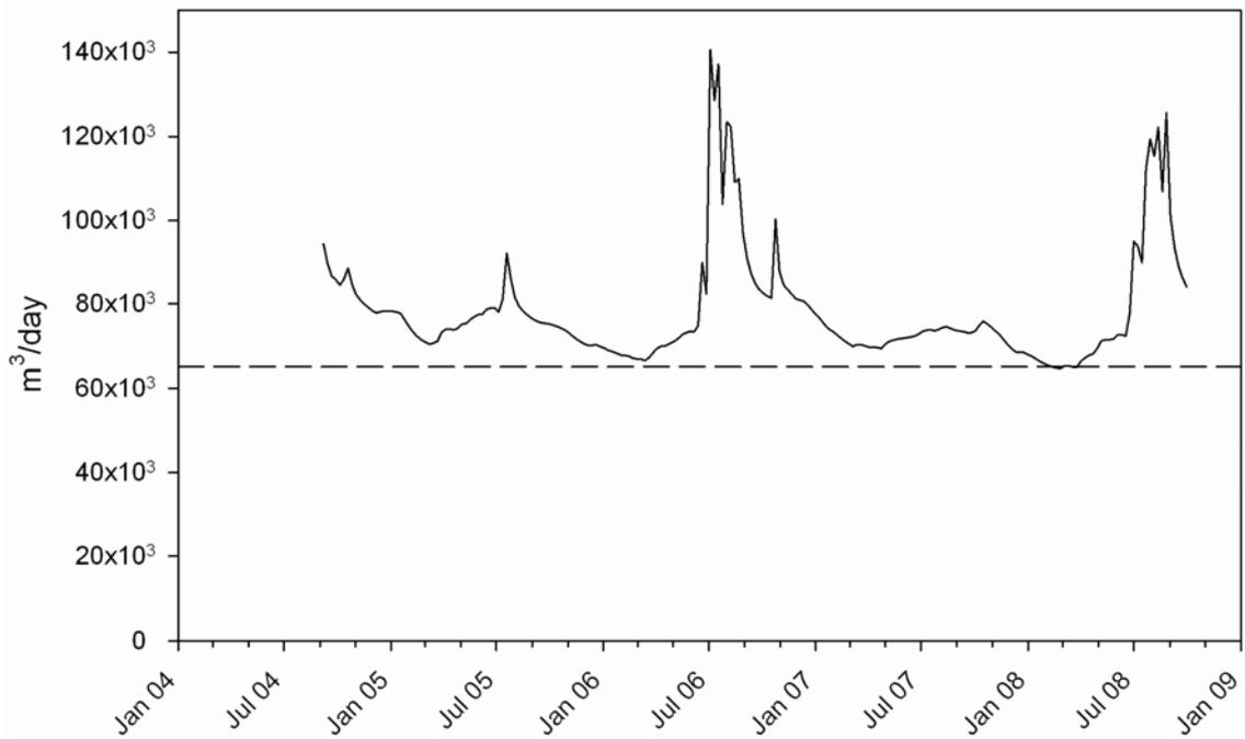
Figure F30: Simulated natural discharge to Stonestead (Dock) Creek when there is no groundwater abstraction. Mean low flow is about 65,000 m³/day (750 L/s) and is indicated by the dashed line.
