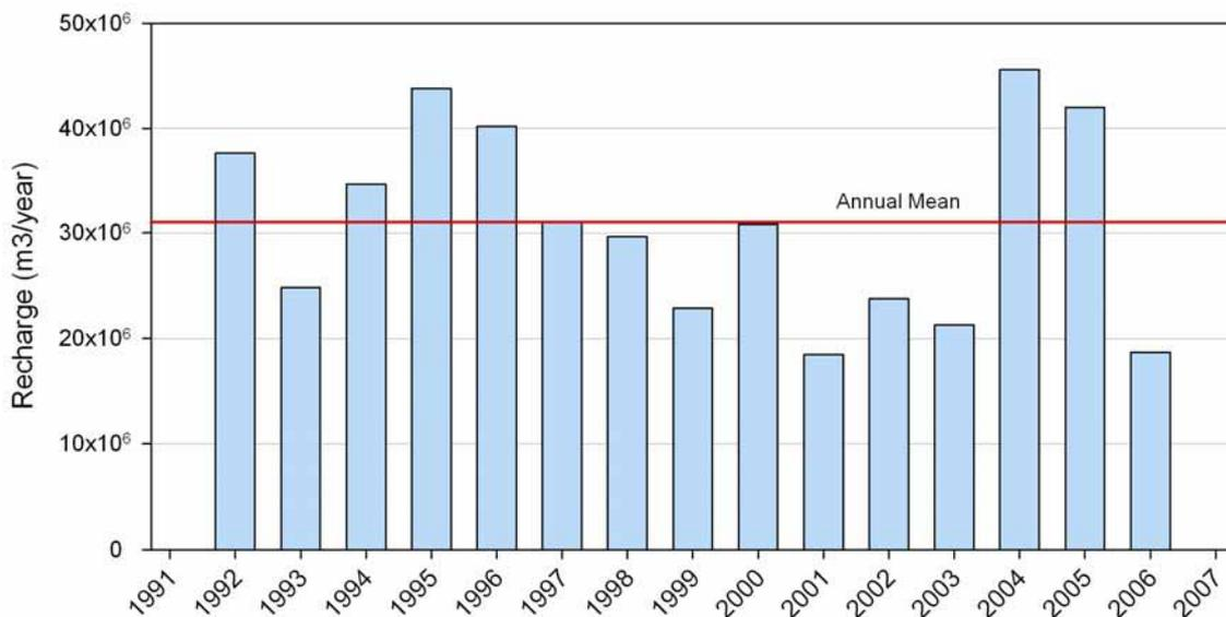
Figure E11: Modelled annual rainfall recharge (1992-2006) for the Mangatarere water management zone (mean recharge equal to  $31 \times 10^6 \text{ m}^3/\text{year}$ )
