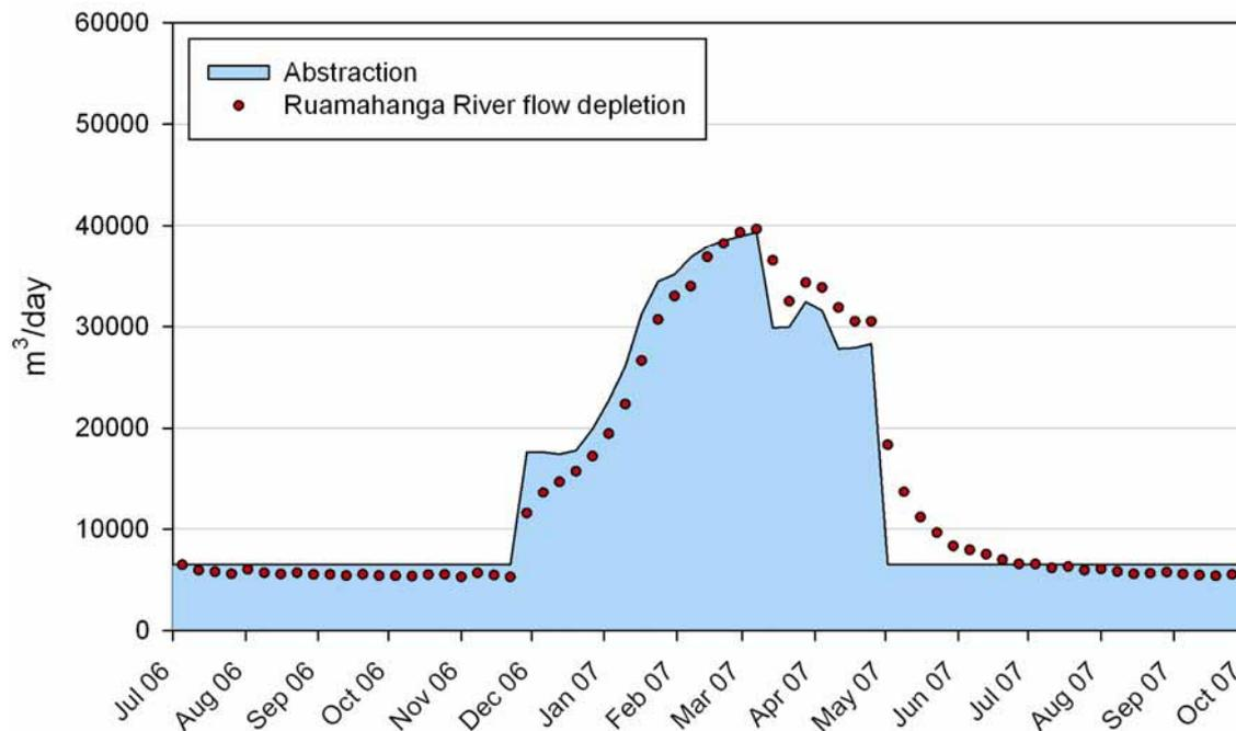
Figure F52: Scenario 1 – Simulated flow depletion in the Ruamahanga River in the Lower Ruamahanga water management zone over the 2006/07 irrigation season, illustrating the high degree of hydraulic connection between the river and aquifer
