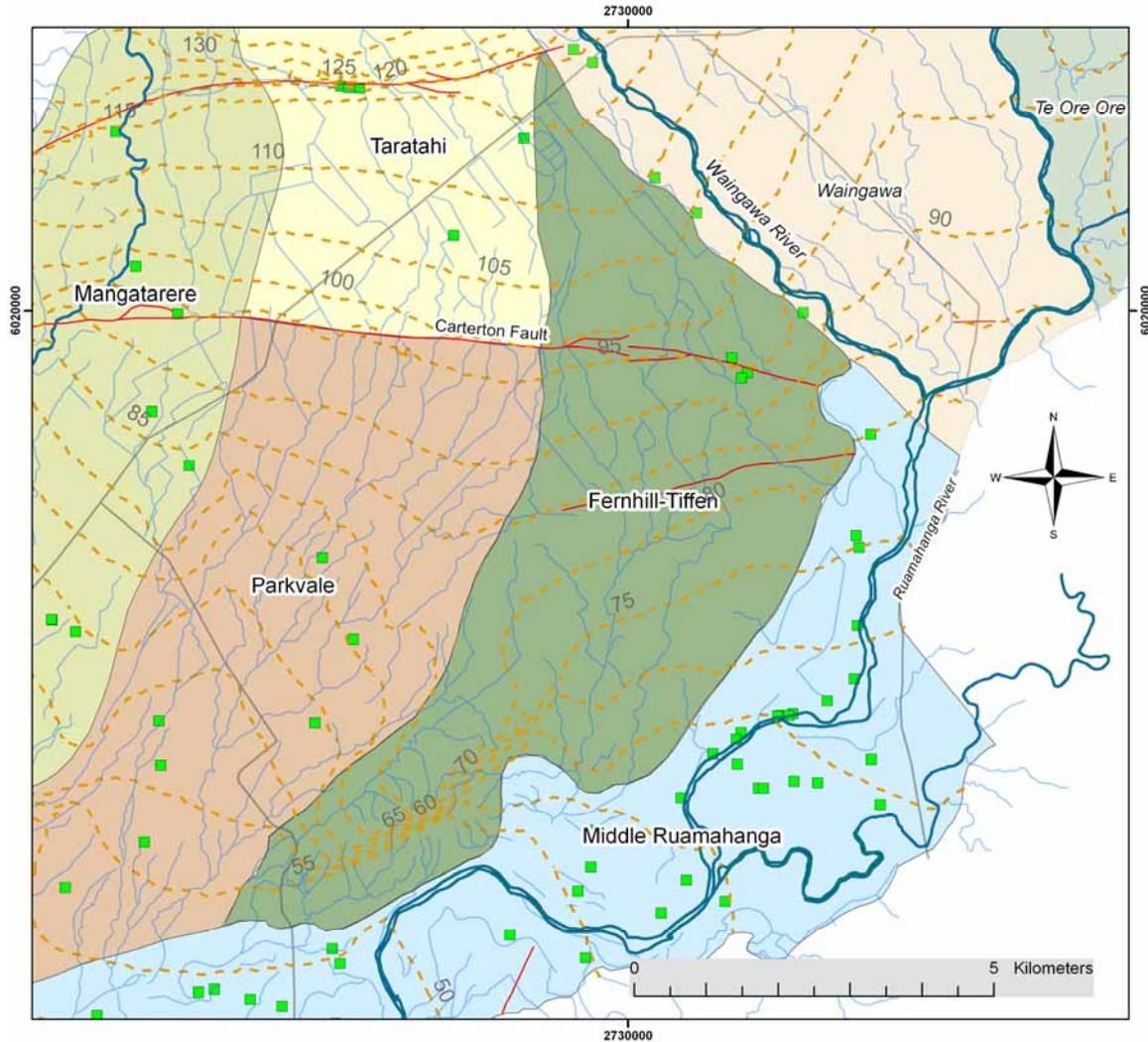
Figure E37: The proposed Fernhill-Tiffen water management zone map showing existing groundwater bores with consented abstraction (green squares) and simulated groundwater flow contours (brown dashed lines at 5 m intervals in metres above mean sea level).
