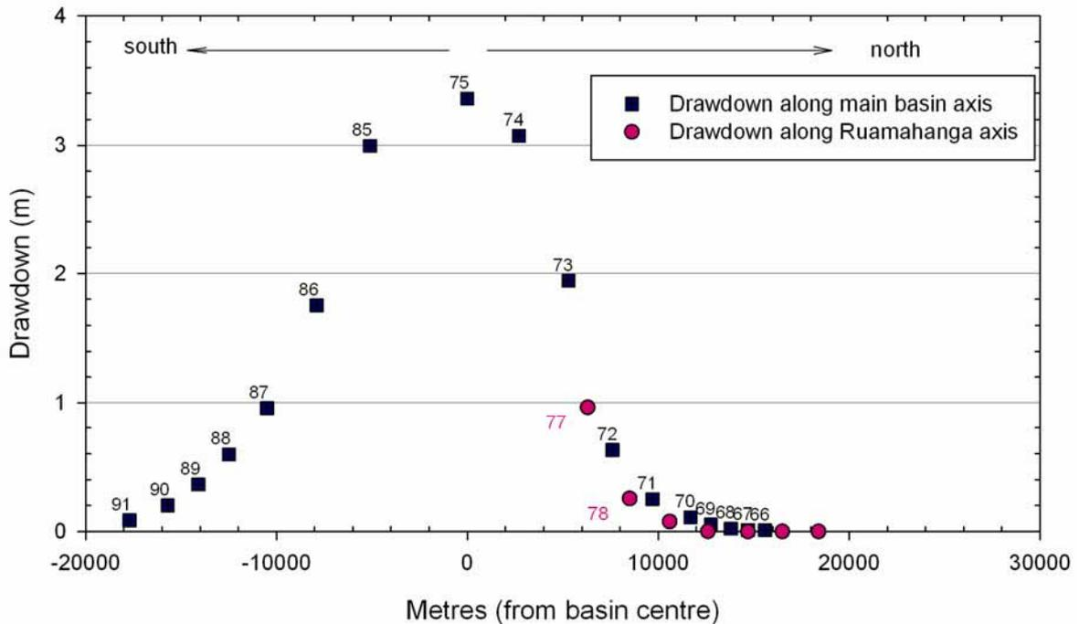
Figure F9: Simulated drawdowns along two axes through the Lake basin in the confined Q2 aquifer associated with a total abstraction of 25,000 m<sup>3</sup>/day. The figure shows the shape of the 'cone of depression' which extends at a shallower angle down-gradient compared to the steep up-gradient profile. Numbered observation points are shown in Figure F8; Point 75 is the centre of the basin – positive meterage to the north and negative to the south of this point.
