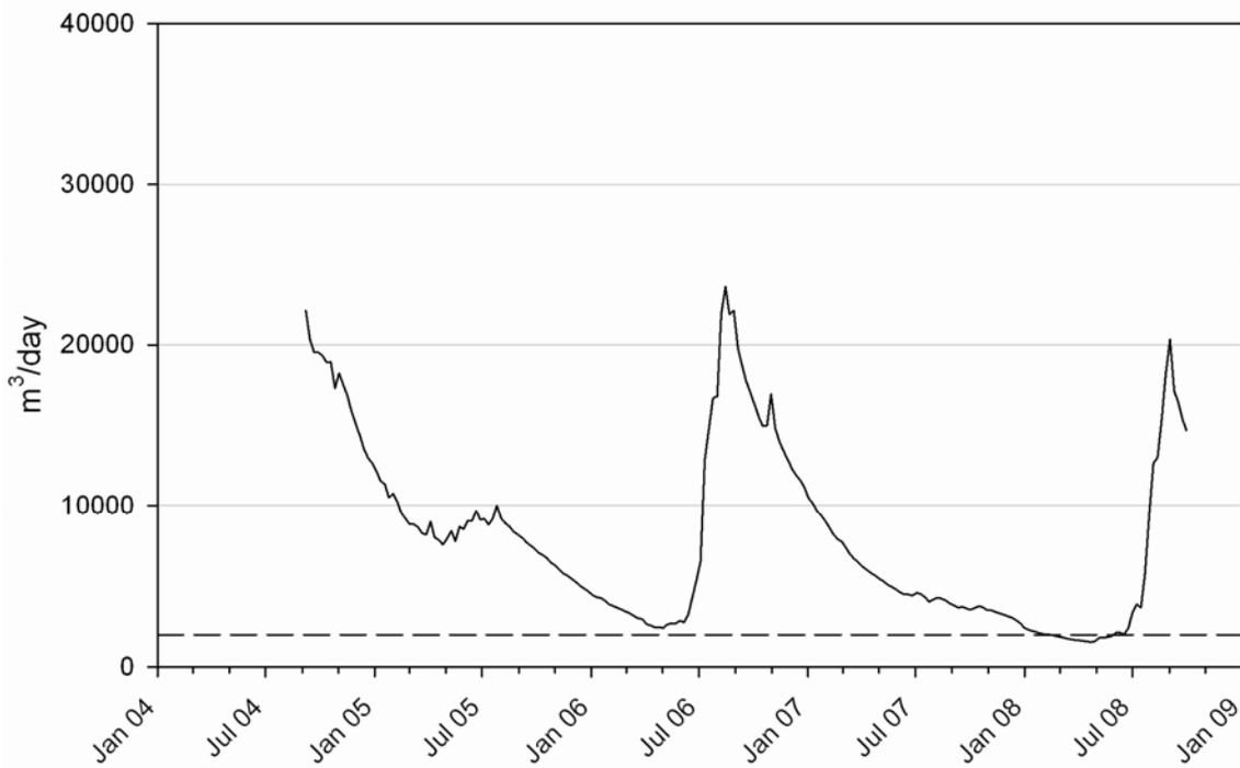
Figure F32: Simulated natural discharge to the Otukura Stream when there is no groundwater abstraction. Mean low flow is about 2,000 m<sup>3</sup>/day (23 L/s) and is indicated by the dashed line.
