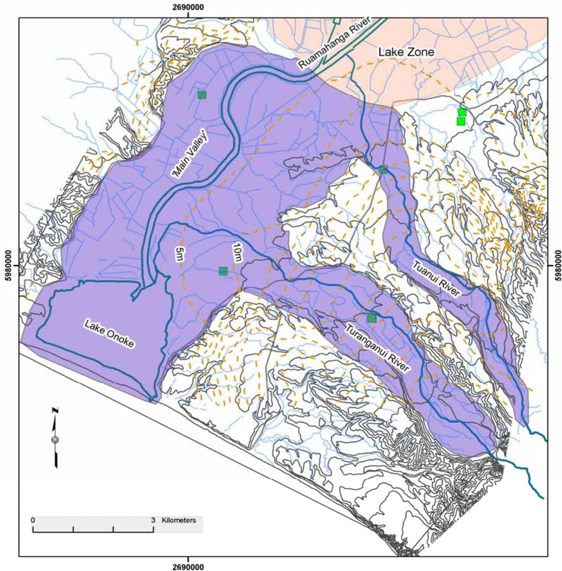
Figure F65: The proposed Onoke water management zone defined by the recent alluvium of the Ruamahanga River valley and the Turanganui and Tauanui side-valleys. The map shows existing groundwater bores with consented abstraction (green squares) and groundwater flow contours (brown dashed lines in m amsl at 5 m intervals).
