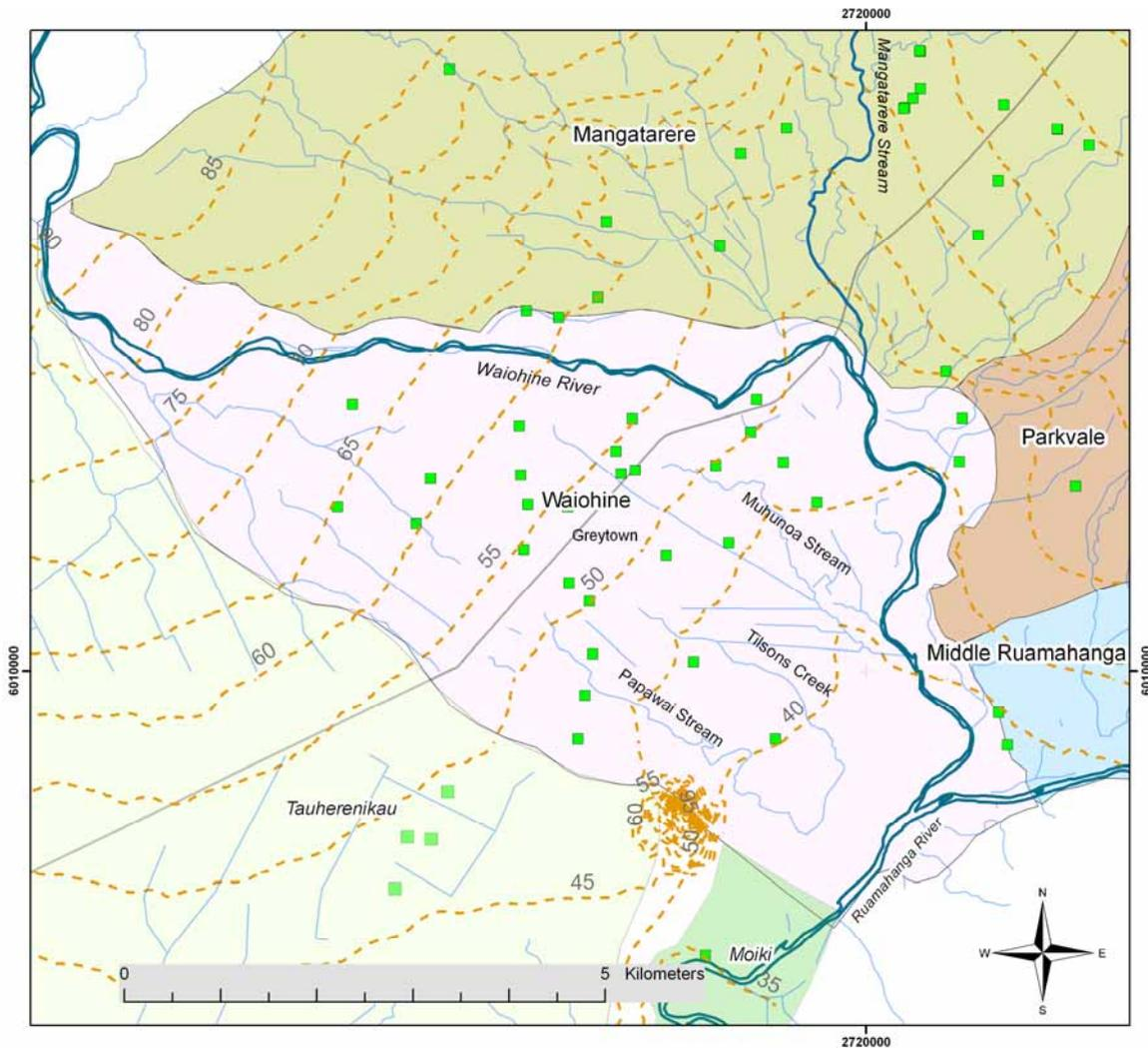
Figure E3: The proposed Waiohine water management zone map showing existing groundwater bores with consented abstraction (green squares) and simulated groundwater flow contours (brown dashed lines, 5 m intervals in metres above mean sea level).
