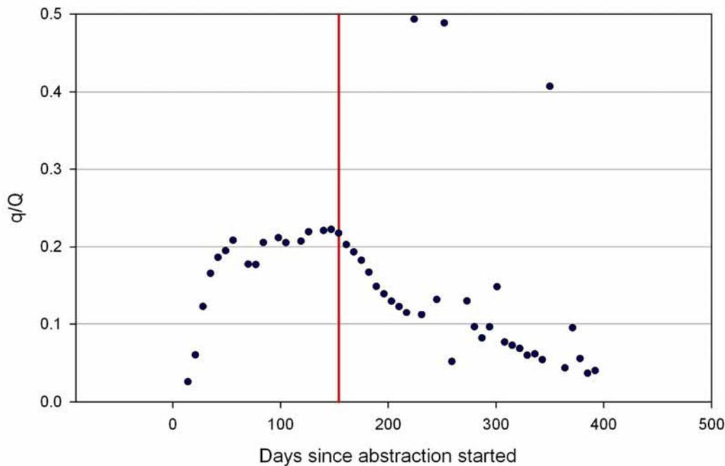
Figure E36: Ratio of spring flow depletion ( $q$ ) to pumping rate ( $Q$ ) for the Taratahi zone scenario resulting from the cumulative effect of shallow groundwater abstraction. The red line shows when groundwater pumping stopped at 154 days at an average rate of 7,300 m<sup>3</sup>/day.
