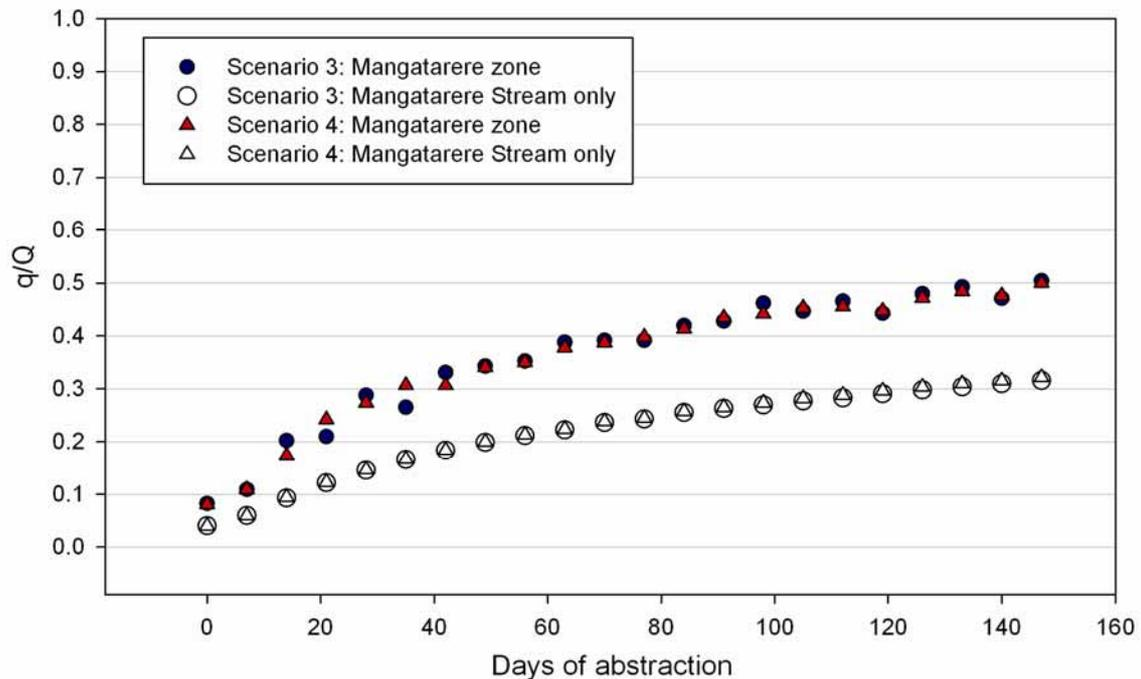
Figure E20: Scenarios 3 and 4 – ratio of surface water depletion ( $q$ ) to pumping rate ( $Q$ ) for both the Mangatarere zone (total depletion for streams and springs) and Mangatarere Stream only – abstraction from semi-confined Q6 aquifer at 12,000 m<sup>3</sup>/day (Scenario 3) and 20,400 m<sup>3</sup>/day (Scenario 4) for 150 days
