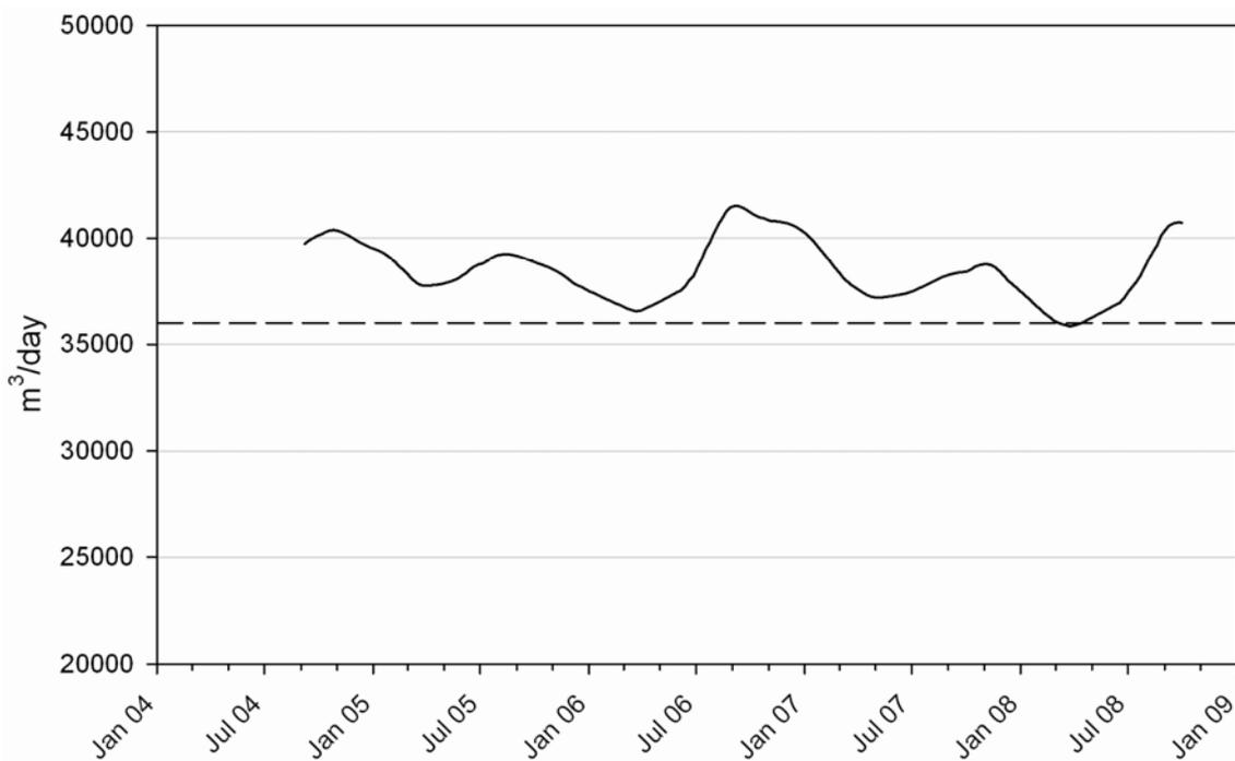
Figure F33: Simulated natural groundwater discharge into Lake Wairarapa when there is no groundwater abstraction. Mean inflow flow is about 36,000 m<sup>3</sup>/day (420 L/s) and is indicated by the dashed line.
