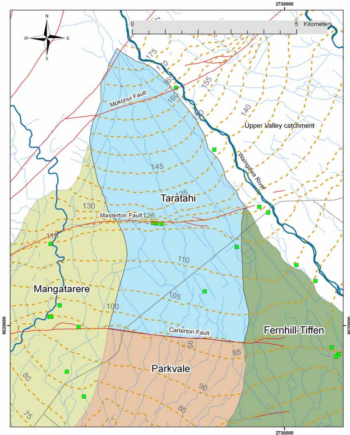
Figure E33: The proposed Taratahi water management zone map showing existing groundwater bores with consented abstraction (green squares) and groundwater flow contours (brown dashed lines at 5 m intervals).
