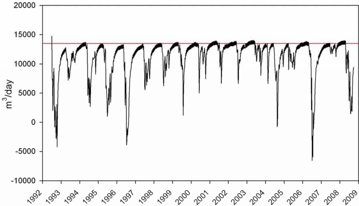
Figure F58: Simulated leakage through the bed of the Dry River, 1992–2008. Mean summer discharge is about 13,000 m<sup>3</sup>/day (150 L/s), shown by the red line.
