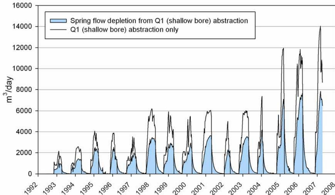
Figure E9: Simulated spring flow depletion (Papawai-Tilsons-Muhunoo) resulting from historic abstraction from Q1 (shallow) bores only in the Waiohine zone. The results show that spring flow depletion is about 60 to 65% of the bore abstraction rate.
