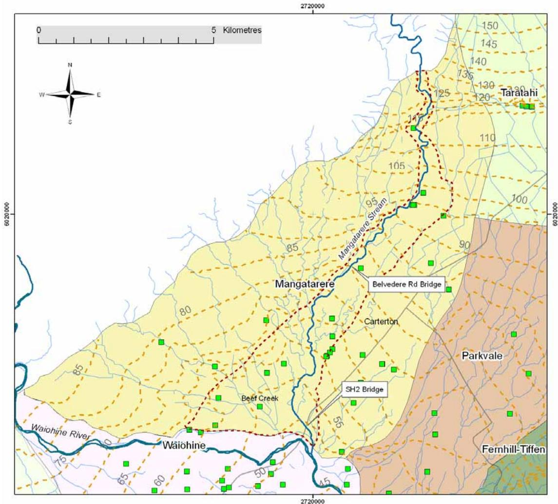
Figure E10: The proposed Mangatarere water management zone map showing existing groundwater bores with consented abstraction (green squares), groundwater flow contours (brown dashed lines, 5 m intervals in metres above mean sea level) and the extent of the alluvial deposits classified as Category A (red dashed line)
