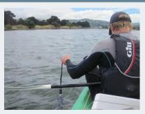
YSI data sonde recording water quality parameters of DO, salinity, chl-a, depth and temperature.
