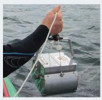
Box core being prepared for deployment (photo above), and retrieved after sample collection (photo below).
