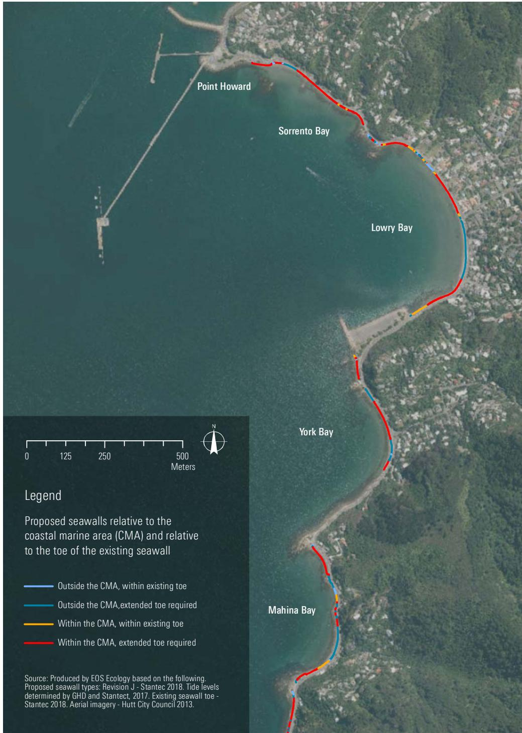
Figure 37 Proposed shared path and seawall works that, once constructed, will extend into the intertidal zone, relative to the existing seawalls (northern extent).
