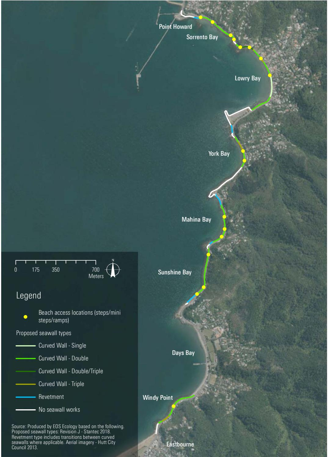
**Figure 2** Proposed seawall treatment types as outlined in the design plans (Revision J) and associated files provided by Stantec 3 September 2018. A more detailed breakdown of the seawall types can be found in Appendix 1.
