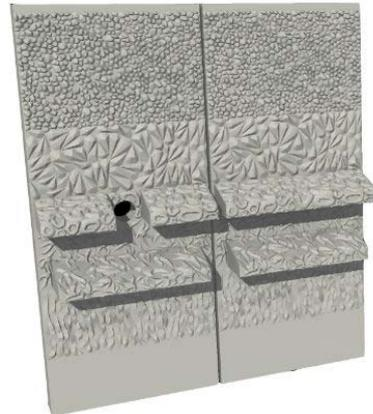
Precast textured concrete panels used to enhance seawall habitat used in the Elliott Bay Seawall Project in Seattle, Washington. Source: <http://www.haddad-drugan.com/seawall-strata> and <https://sdotblog.seattle.gov/2014/04/23/more-than-just-a-seawall-enhancing-habitat-in-elliott-bay-and-preserving-public-safety/>
