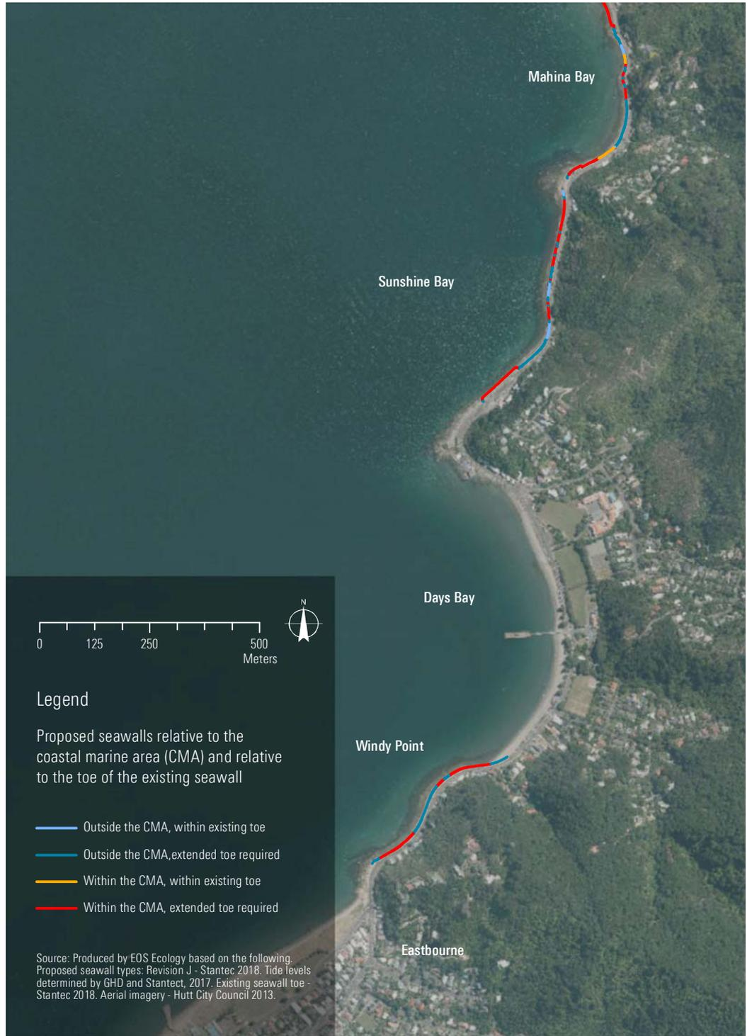
**Figure 37** (cont.) Proposed shared path and seawall works that, once constructed, will extend into the intertidal zone, relative to the existing seawalls (southern extent).
