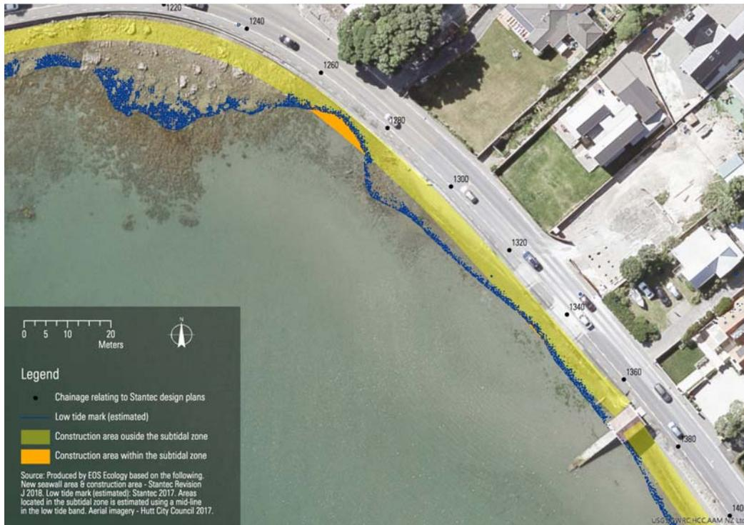
Northern Lowry Bay (around chainage 1260-1360). Treatment type: double or triple curved wall
