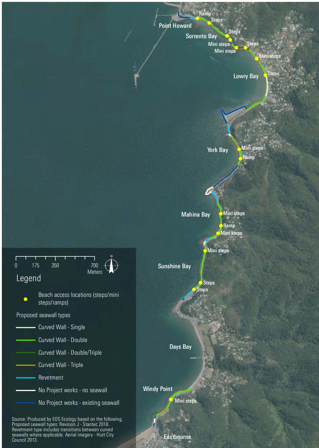
Figure 34 Proposed seawall types as outlined by the Design Plans and associated files (Revision J) provided by Stantec on 3 September 2018. Further breakdown of the curved seawall and access types is provided in Appendix 1.
