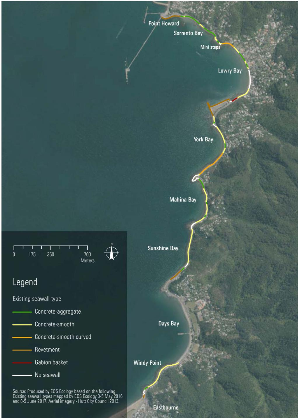
Figure 6 Categories of the seawalls that currently exist along the Eastern Bays shoreline as determined during surveys by EOS Ecology on 3-5 May 2016 and 8-9 June 2017.
