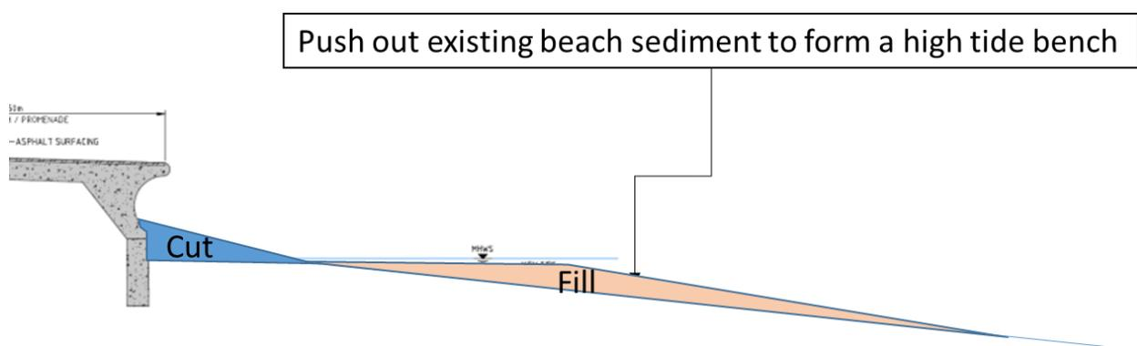
Figure 6-1 Sketch showing initial high tide bench formation moving existing beach material from the upper beach to the lower beach
