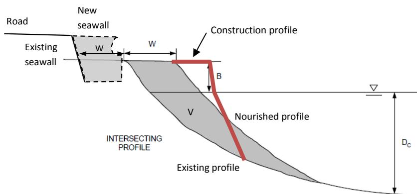
**Figure 2 Schematic of beach construction profile using “overbuilding” method [Not to scale]**
