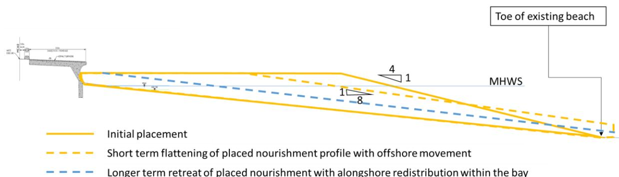
Figure 6-2: Illustration of sand nourishment placement and expected cross shore redistribution and landward retreat of the placed profile due to the alongshore processes
