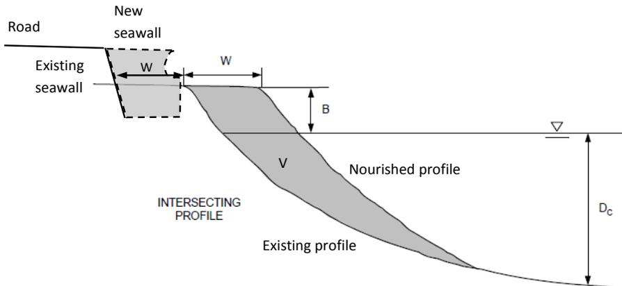
**Figure 1 Schematic of beach nourishment as cross section through beach [not to scale]**
