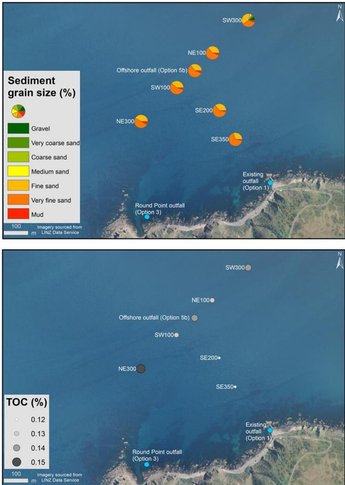
Figure 10. Sediment grain-size composition and concentration of organic carbon (TOC) in sediments at the seven grab-sampling stations. Concentration categories are based on ‘natural breaks’ that best group similar values and maximise differences among classes.
