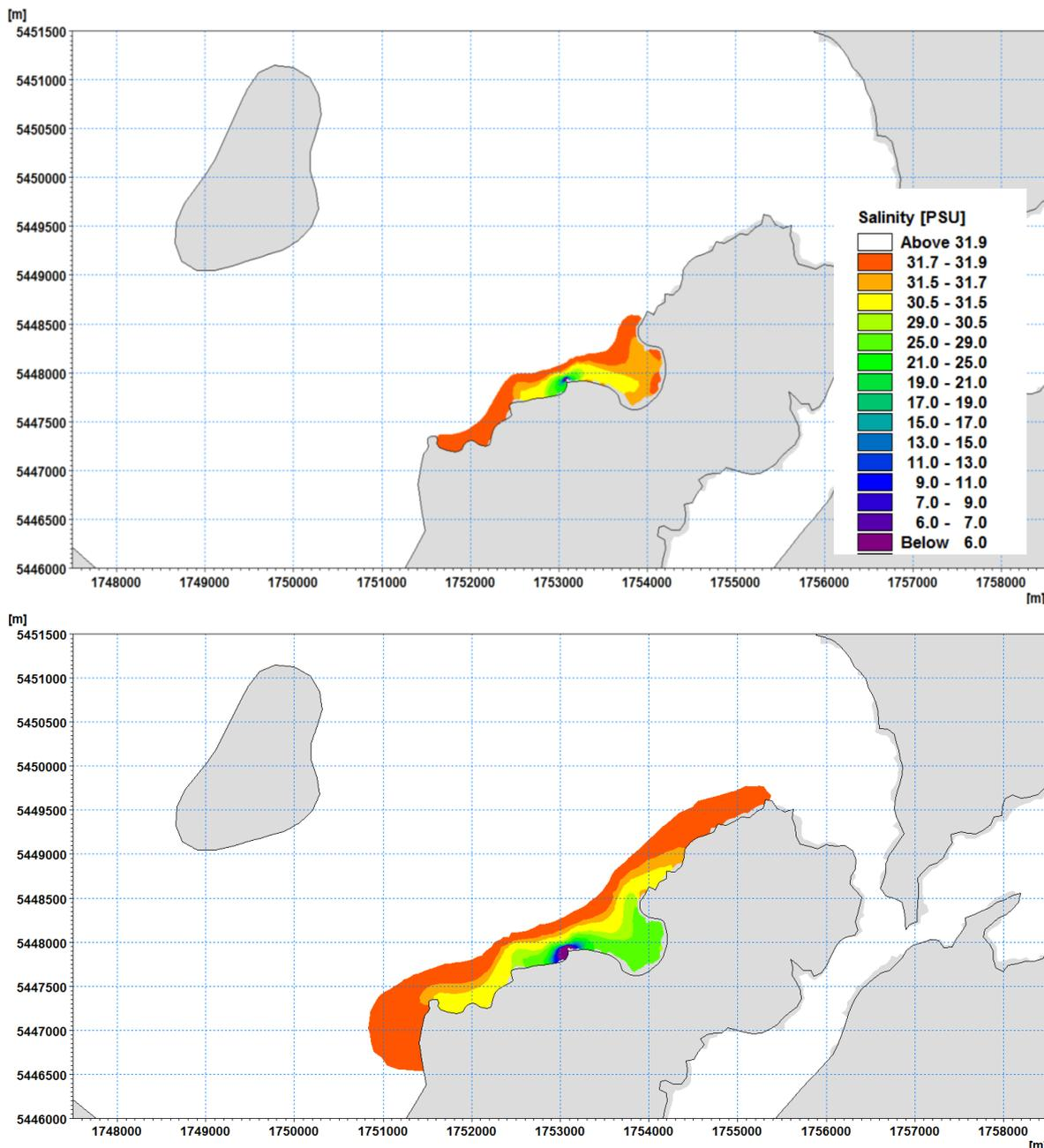
Figure 16. Predicted mean salinities for the average discharge rate from the existing Porirua WWTP discharge (300 L/s: upper figure) and for the design discharge rate (1500 L/s). Source: DHI (2018).
