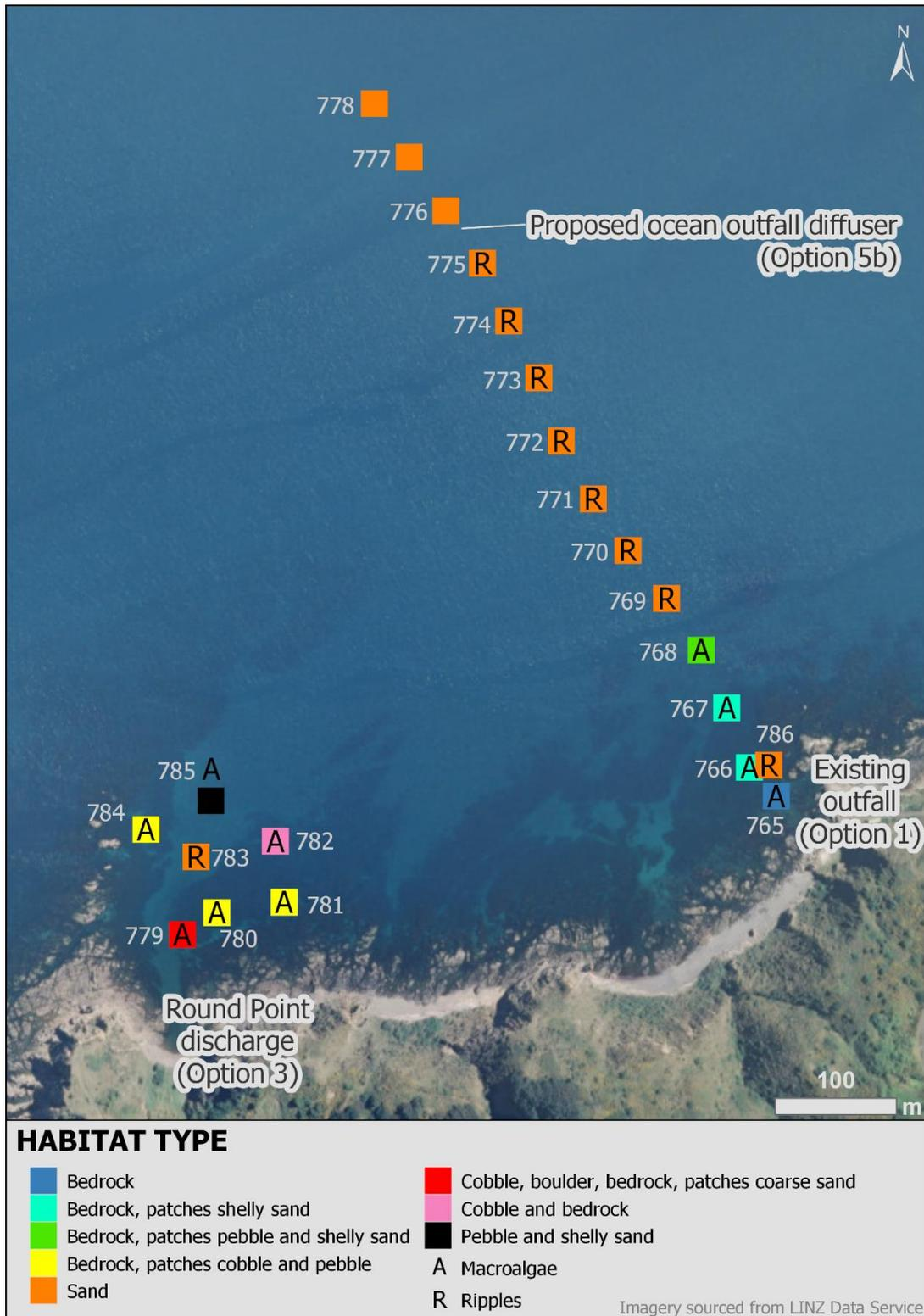
Figure 5. Seabed habitats identified from drop-camera videos. In addition to substratum type, the presence of macroalgae (A) on hard substrata, ripples (R) in sandy areas, and the way-point numbers are also shown.
