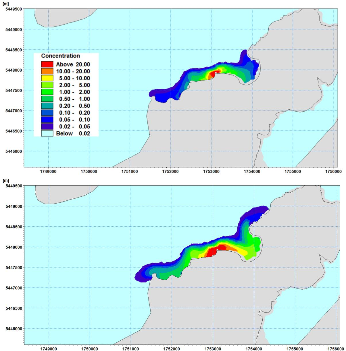
Figure 17. Predicted median concentration of wastewater for the average discharge rate from the existing Porirua WWTP discharge (300 L/s: upper figure) and for the design discharge rate (1500 L/s). Source: DHI (2018).
