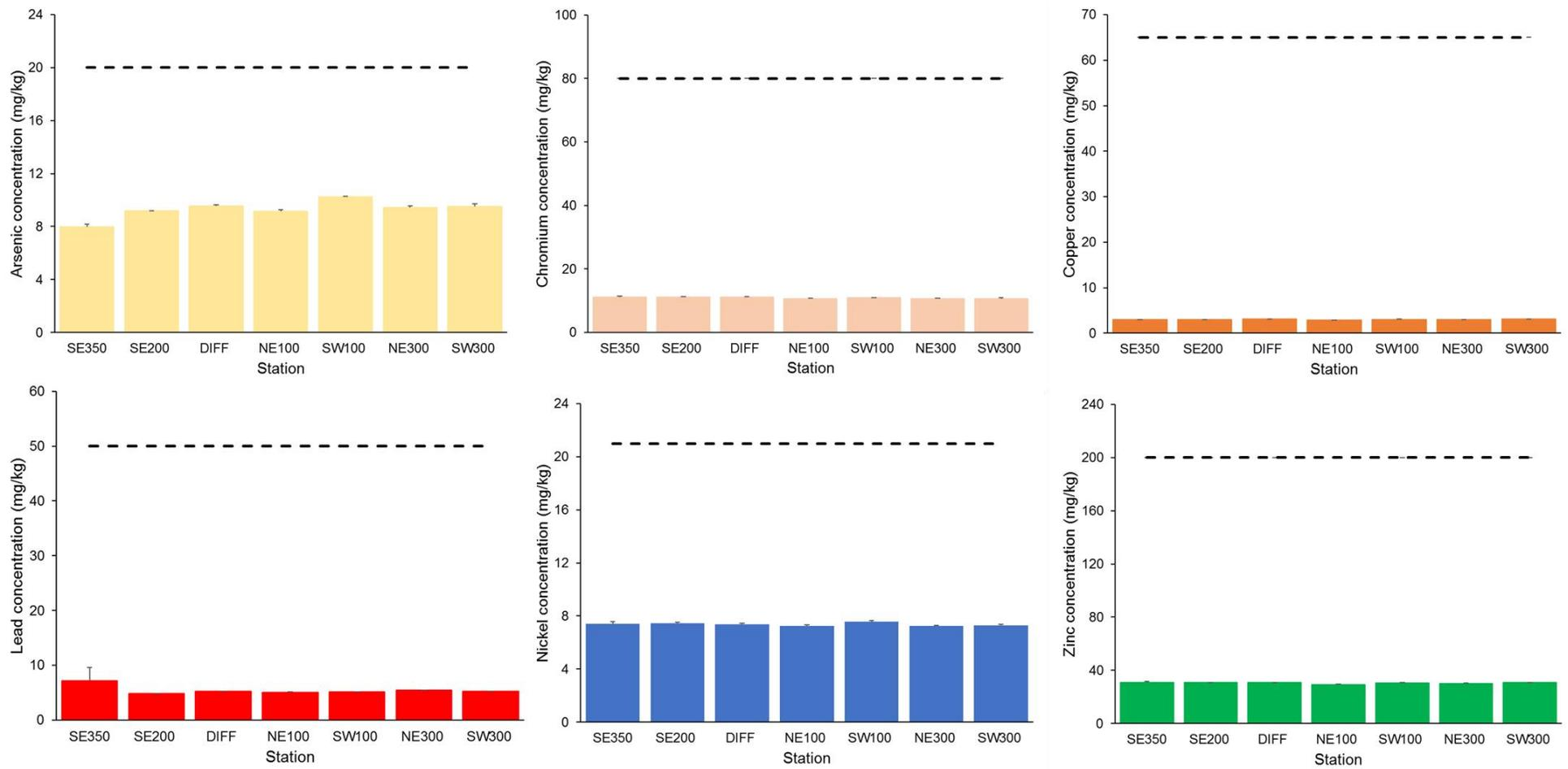
Figure 11. Concentrations of trace metals in sediments at the seven grab-sampling stations. Values are means ( $\pm$  SE) of three replicates. Dotted lines represent the ANZG (2018) default guideline values for sediment quality. Note different y-axis scales for different determinands.
