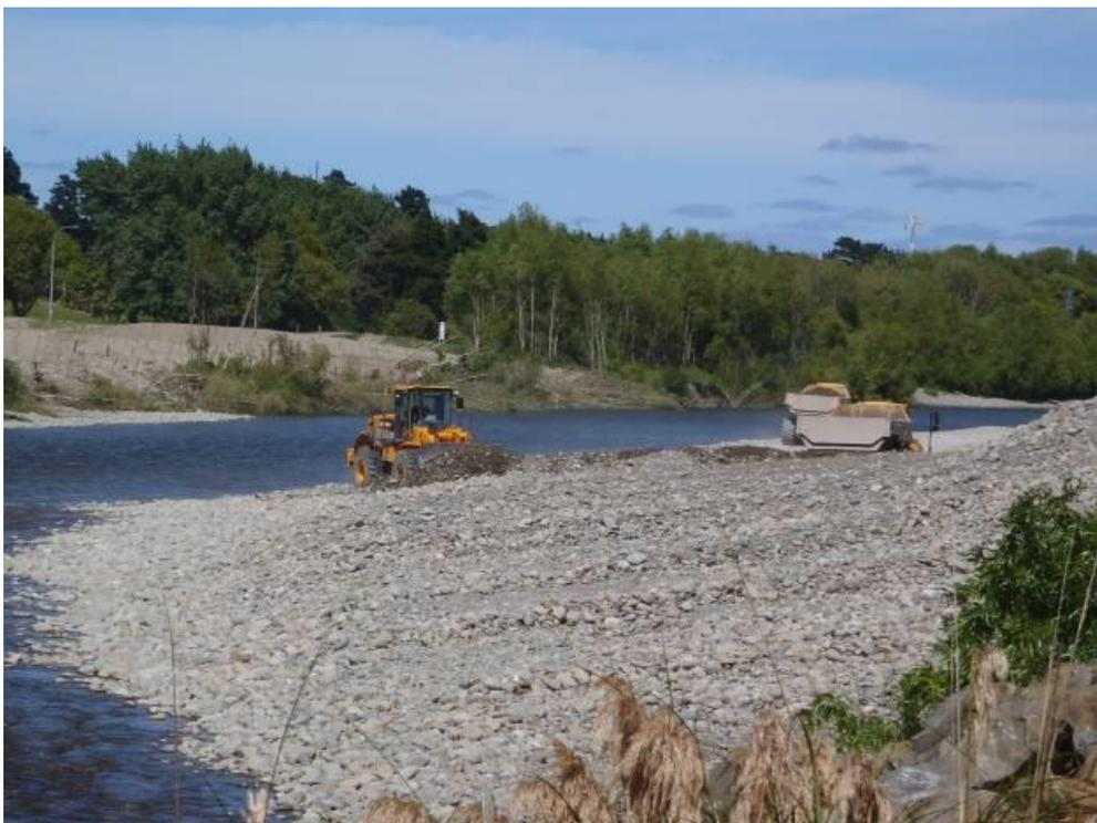
*Figure 11: Gravel extraction: front-end loader loading an off-road dumper truck*
