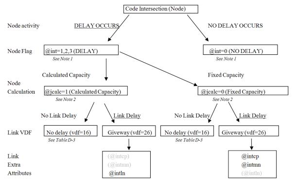
Figure 2-10: Intersection Coding Flow Chart
