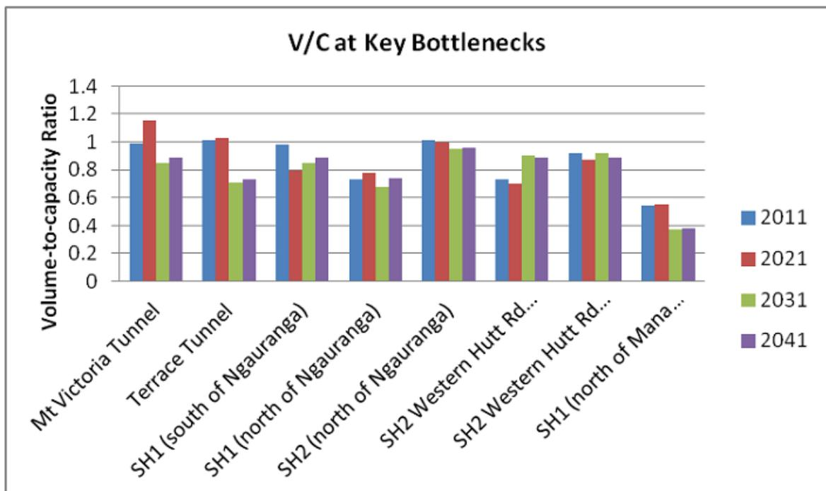
**Figure 4-5: Volume-to-capacity Ratios at Key Bottlenecks, AM Peak**
