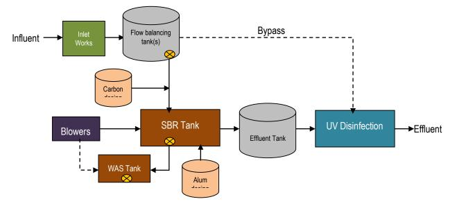
Figure 13: Process flow diagram for Sequencing Batch Reactor process
