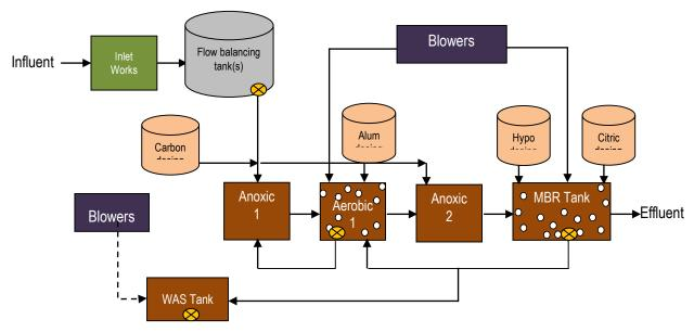
Figure 14: Process flow diagram for membrane bioreactor process
