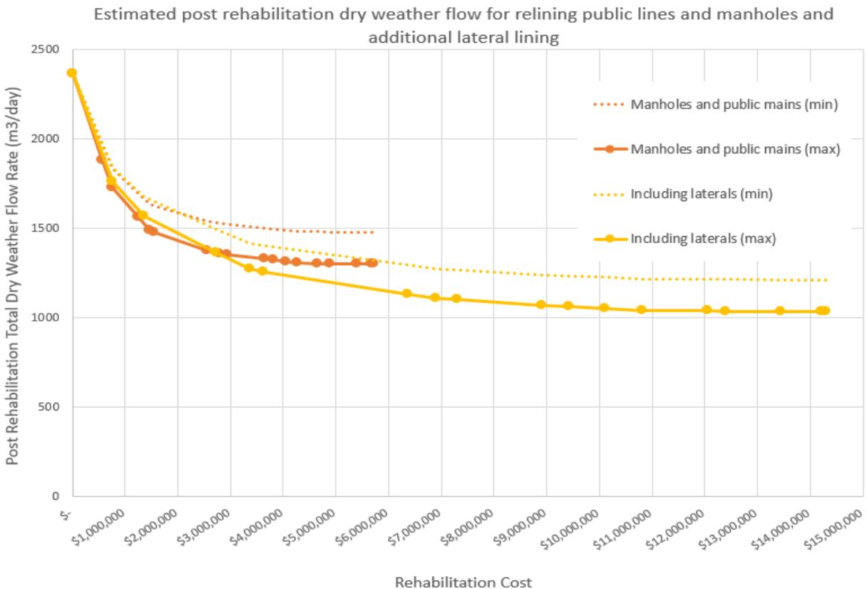
Figure 7: Cumulative costs and post rehabilitation dry weather flow
