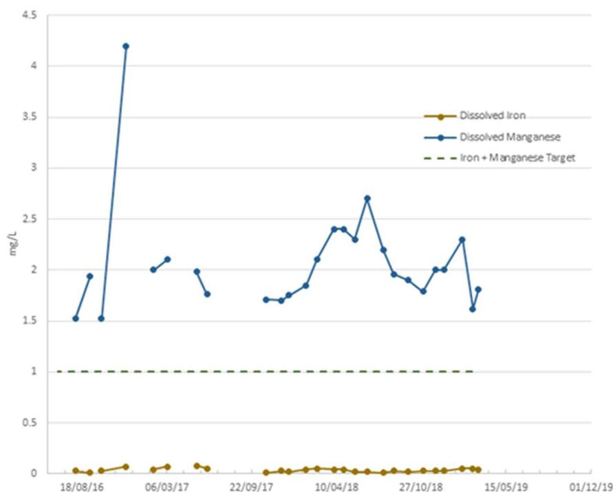
Figure 2: Dissolved Fe and Mn monitoring results (between June 2012 and July 2019) at the site ‘TTD’ located about 80 m below the wetland outlet
