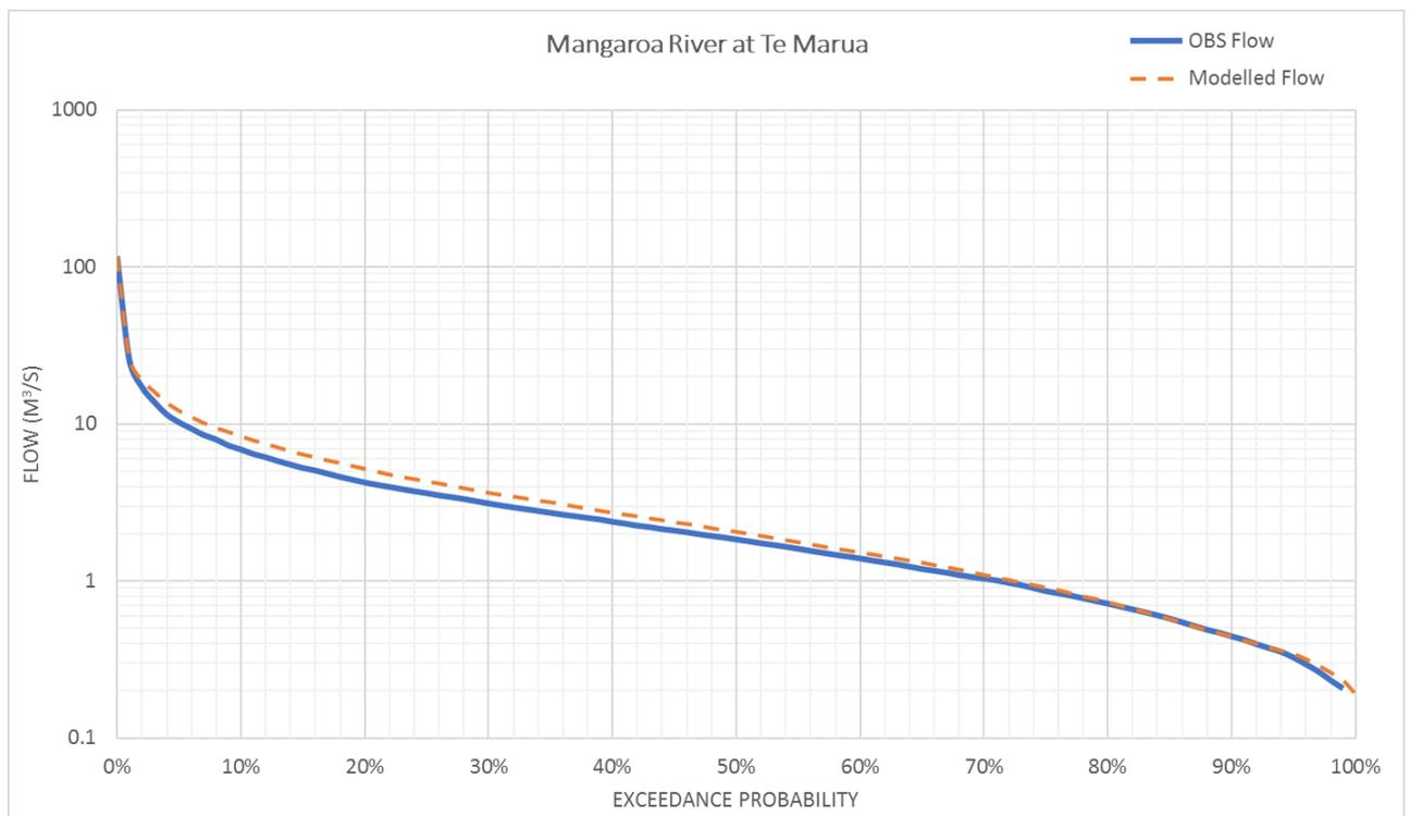
Figure 3 Flow duration curve for Mangaroa river at Te Marua
