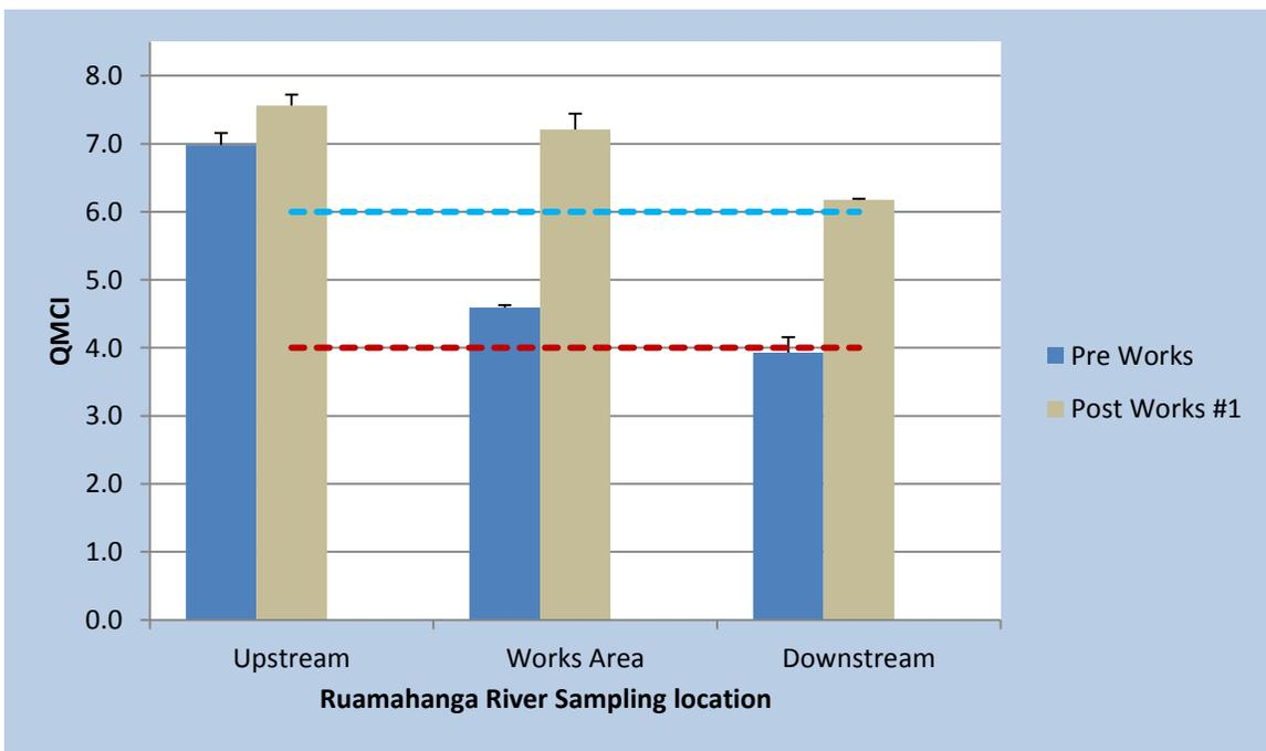
**Figure 41:** Mean ( $\pm 1$  SE) A. MCI and B. QMCI for sites sampled on the Ruamahanga River in relation to river works undertaken by GWRC in 2013. Thresholds indicative of good water quality are plotted as a blue dashed line and those of poor water quality as a red dashed line. (Refer Table 3).
