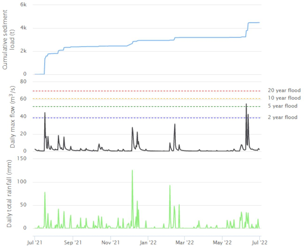
Figure 5: Pāuatahanui Stream at Gorge cumulative sediment load, daily maximum flow and daily total rainfall for the 2021/22 monitoring season. Sediment load is predicted using a turbidity vs discrete suspended sediment concentration model that is updated annually, see [Morar & Alberto \(2018\)](#) for more information. The flow event lines represent the flow level at which we would expect  $n$  years before another event that size.
