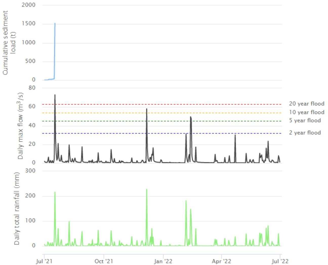
Figure 3: Porirua Stream at Town Centre cumulative sediment load, daily maximum flow and daily total rainfall for the 2021/22 monitoring season. Sediment load is predicted using a turbidity vs discrete suspended sediment concentration model that is updated annually, see [Morar & Alberto \(2018\)](#) for more information. The flow event lines represent the flow level at which we would expect  $n$  years before another event that size.
