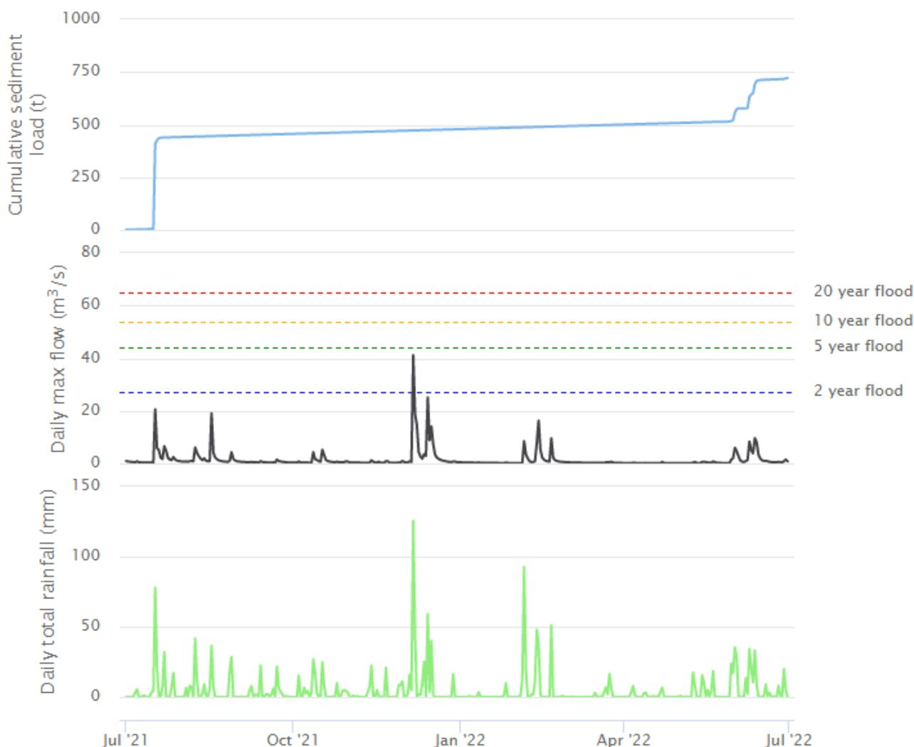
Figure 4: Horokiri Stream at Snodgrass cumulative sediment load, daily maximum flow and daily total rainfall for the 2021/22 monitoring season. Sediment load is predicted using a turbidity vs discrete suspended sediment concentration model that is updated annually, see [Morar & Alberto \(2018\)](#) for more information. The flow event lines represent the flow level at which we would expect  $n$  years before another event that size.
