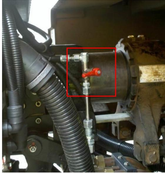
Figure B-44 Pneumatic circuit isolation cock (closed position)
