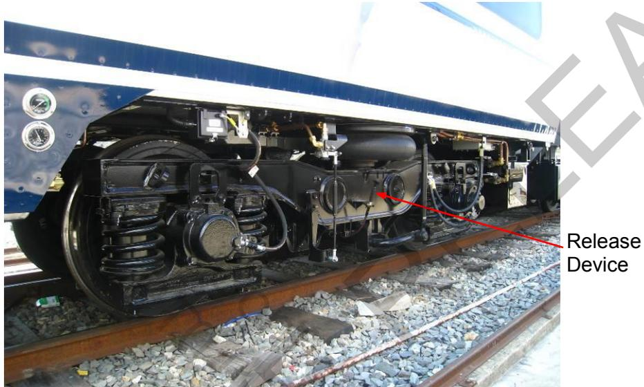
Figure B-5 Release Device on Motor Bogie
