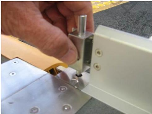
Release button to deploy side rail
