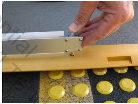
Push pin down to lock side rail in place
