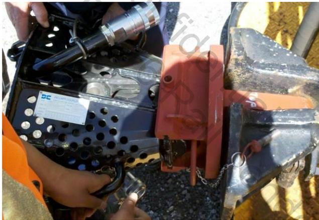
Figure B-49 Fitting rescue adapter to hook & pin locomotive
