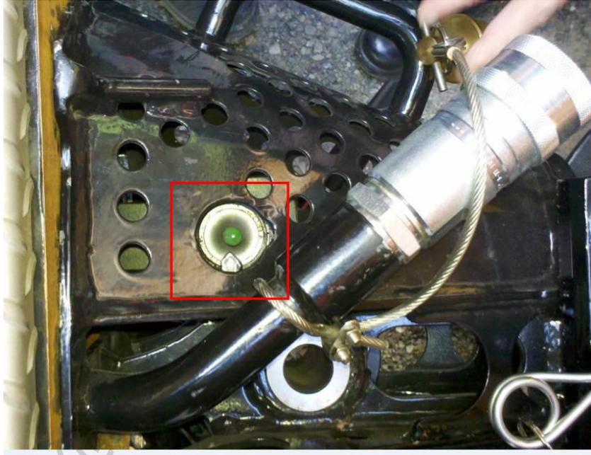
Figure B-51 Rescue adapter successfully coupled
