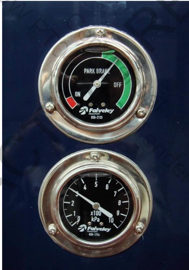
Figure B-7 External Park Brake and BC Gauges Applied/ Released
