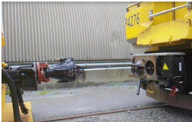
Figure B-50 Rescue adapter assembled on locomotive
