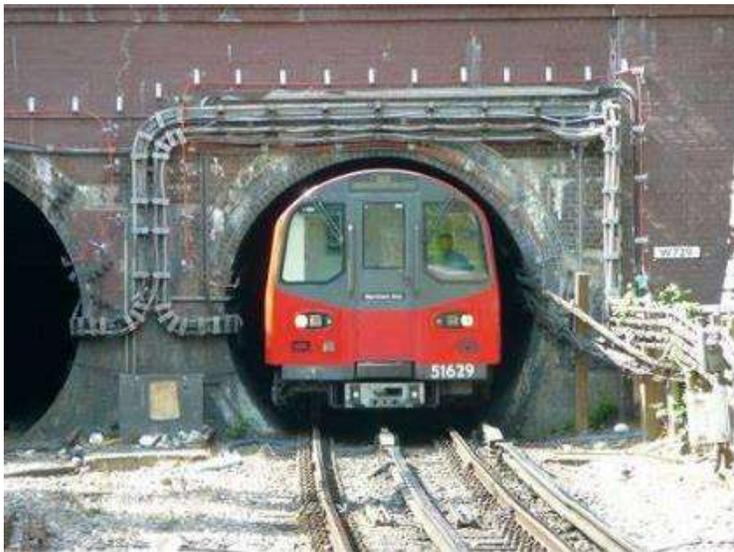
Figure 28: Example of vehicle modified to fit through tunnel
