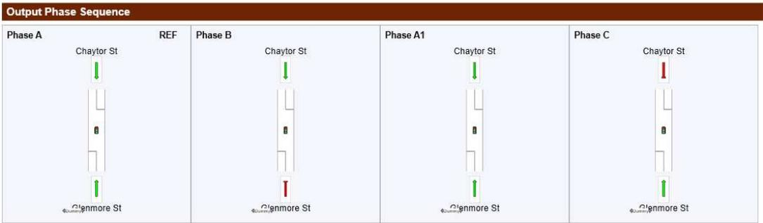
Figure 16: Phase sequence for Option 1h, partial one-way operation of the tunnel
