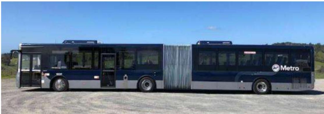
Figure 29: Example of an articulated bus
