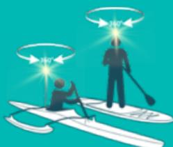
Boats less than 7 metres long and not capable of more than 7 knots (including kayaks and paddle craft) may carry navigation lights or display a 360° all-around white light when in Wellington or Porirua harbours.
