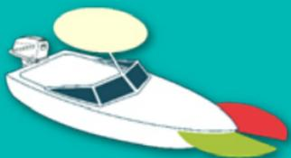
When underway, powerboats less than 12 metres long may combine their stern and masthead lights into a single all-round white masthead light. The boat should also have red and green sidelights.
