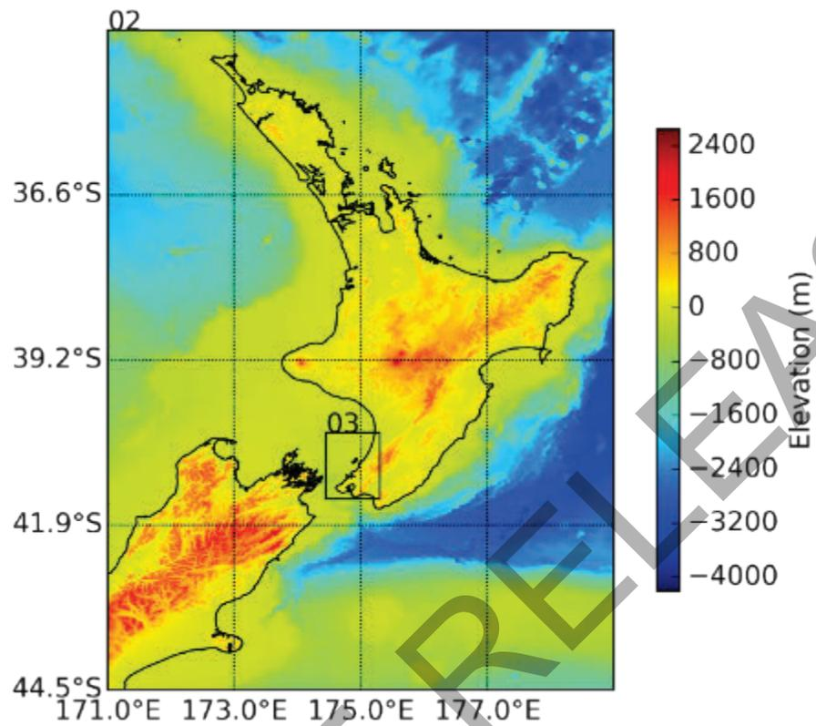
**Figure 2.2** Nested grid setup for tsunami generation and propagation modelling. This figure shows the nested grid layers 02 (full extent of the map) and 03 which both focus on New Zealand and offshore regions at increasing levels of detail. Elevation above sea level is colour-coded in metres.
