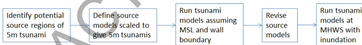
**Figure 3.6** Outline of scheme for Orange Zone calculation. The scheme shown here is for developing a zone capable of encompassing a 5m tsunami. MSL = Mean Sea Level, MHWS = Mean High Water Springs ('high tide').
