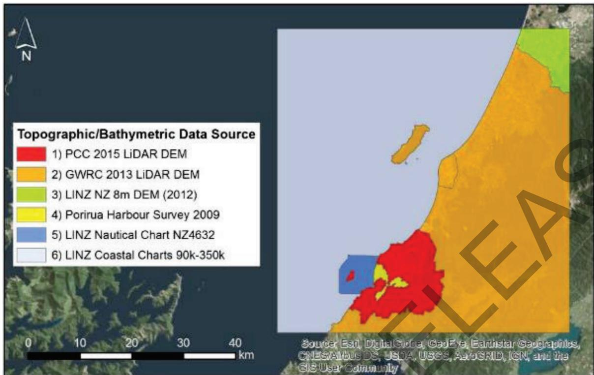
**Figure 2.5** Data sources for the grid layer 04 DEM: Polygons outline the areas for different data sources that were used to construct the DEM (see legend). Sources 1, 2, and 3 refer to the topographic (land elevation) data and sources 4, 5, and 6 to the bathymetric data.
